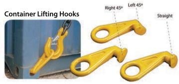
Use what the pros use to lift sea containers. These Container Hooks were developed to be used on the corner eyes of a sea container during a direct lift. They are available in left and right versions for using as a sling or a 90 degree version for direct lifting. These are designed for lifting purposes only.
