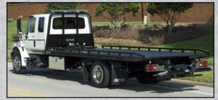
When mounted on most air ride chassis, with the air dumped, the 16 series L.C.G. has lower then an 11° load angle, making it ideal for loading low clearance vehicles or equipment without using ramps or wood.
