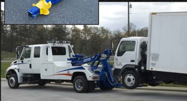
The 2465 comes standard with a low-profile crossbar with removable ends, one set of lift forks, fork holders and a 6,000-lb. pivoting L-Arm System.
