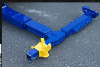
The 2465 comes standard with a low-profile crossbar with removable ends, one set of lift forks, fork holders and a 6,000-lb. pivoting L-Arm System.
