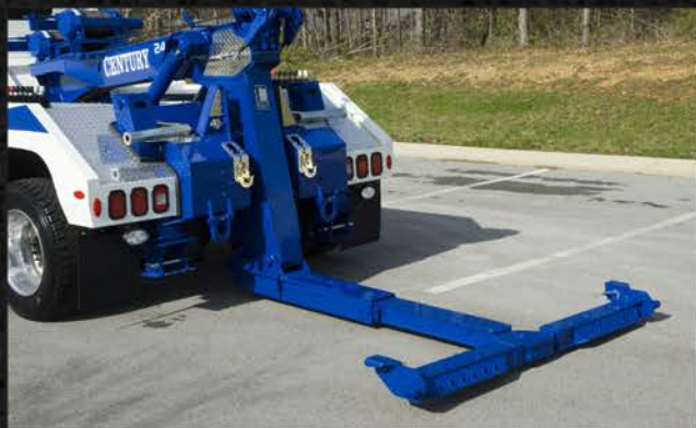
The fabricated underlift is rated at 7,000 lbs. lift capacity at its fully extended reach using lifting forks and has a tow capacity of 20,000 lbs. This makes the Century 2465 ideal for towing a wide variety of light- and medium-duty trucks, as well as automobiles.
