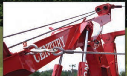
The 3212 G2 allows the cable to run through a snatch block and hooked to a clevis at the base end of the boom for side pull applications.
