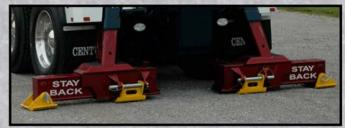
The optional rear stabilizers, similar to those used on Century Rotators, provide hydraulic horizontal extension of up to an additional 48" of stance when extended for extreme side pull recoveries.
