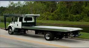
As the cost of fuel, parts, labor and general maintenance increases you need to maximize your equipment's payload per mile. Century's 3-Car Carrier combines a 10 Series Steel or Aluminum carrier and wheel lift with an over-the-cab rack for the perfect package in multivehicle hauling.
