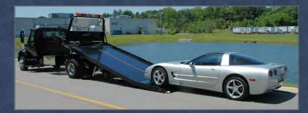
The Right Approach option available on Century 10 series steel carriers eliminates the need for wood planks or ramps when loading and unloading low clearance vehicles. The release handle allows the rear hinged deck section to be lowered to a 6° load angle. A removable cable guide is inserted in the deck to keep the cable low while winching the vehicle onto the rear deck.
