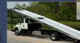
After the vehicle's front wheels are on the carrier, the deck can be leveled out and the cable guide removed allowing the vehicle to overcome the second clearance problem with the forward section of the deck. With the front wheels on the front section of the deck the process can be repeated again to eliminate clearance problems such as low exhaust or extended rear overhang.
