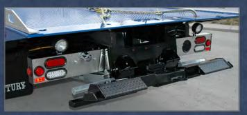
The low profile fabricated wheel-lift stinger provides 68" of reach. When retracted the crossbar is tucked in close to tailboard with minimal overhang. Century's 3-Way Pivoting L-arm System or the popular AutoGrip II crossbar is also available.
