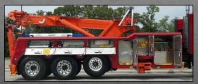
Century's aluminum body is designed to optimize space for your lift forks and popular towing and recovery equipment. Optional front tunnel saddle boxes are available in a variety of sizes to meet your specific equipment needs. All Century Heavy-Duty bodies come with an aluminum tread-plate walkway for easy access to the center section of the recovery unit.
