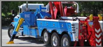
The Century RXP option for the 1140 tri-axle rotator incorporates dual 35,000-lb., two-speed planetary winches, as well as 212" of spread for more stability when lifting. The RXP also provides additional front-axle weight for towing heavier loads and gives operators countless rigging possibilities for those difficult recoveries, thanks to the two additional winches.
