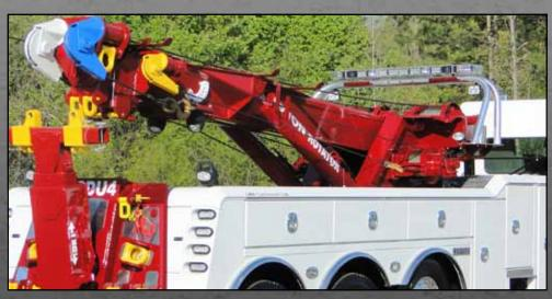
Dual 15,000-lb. turret-mounted winches are optional on the Century 1140 Rotator and come with additional sheave heads mounted on the side of the outer boom, two 175' lengths of 1/2" wire rope and two 5-ton alloy swivel hooks.
