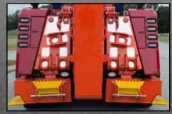
The rear outriggers on Century Rotators were redesigned with a 2½° angle and are now fitted with new lighter-weight spade attachment that is easily stored on the rear legs. The user-friendly spade
