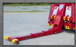
The LDU is standard on both the 1130 and 1140, and provides 139" of reach with a lift capacity of 15,000 lbs. when fully extended. Fully retracted, the LDU has a reach of 55" and a lift capacity of 35,000 lbs.
