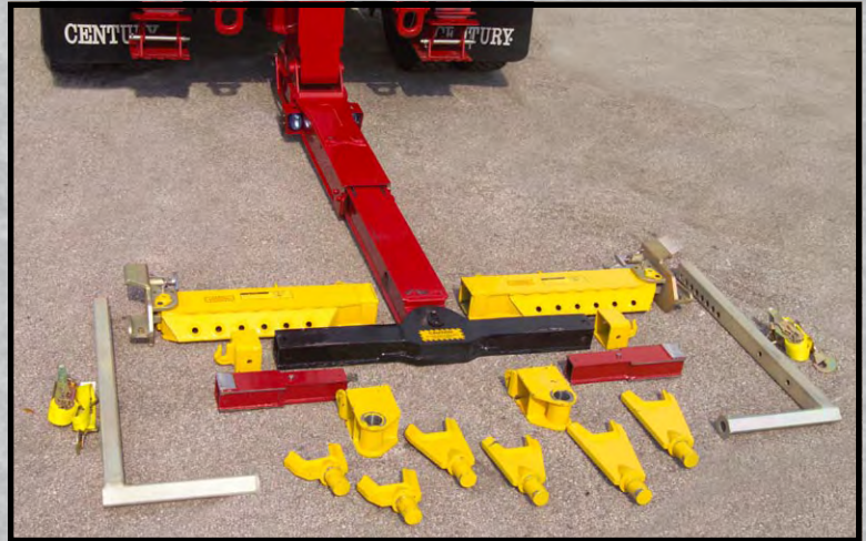
The 3212 comes standard with a low profile crossbar with removable ends, 3 sets of lift forks, fork holders, and 6,000 lbs. pivoting L-Arm System.
