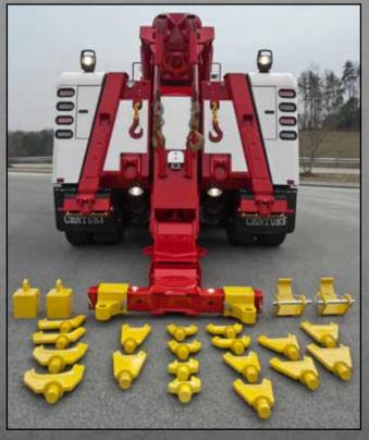
Standard equipment includes 9 sets of cast forks, pivoting spring lift adaptors, chain hook end cups and low profile cast forks holders to provide you with the attachments you need for most towing applications. Century provides the largest choice of standard and optional forks and attachments in the industry.
