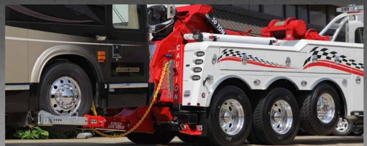
To provide you with the strength and durability you need for your toughest tows while still providing the lowest profile stinger to get under those extremely low vehicles, Century offers the Low Rider Underlift. Constructed using four plate high tensile steel design and available on both the 7035 & 9055. The "Street" Low Rider provides you with the standard reach while the "Coach" Low Rider provides additional reach to haul those difficult pumpers, packers, coaches, and fire trucks.
