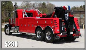
The 5230 is designed to be the ideal unit for towing when scale weight is an issue. The 5230 provides 113" of underlift reach to easily handle most vehicles and is standard with Century's weight-saving aluminum body. A 30-ton recovery boom and 25,000 lb. winches completes this popular package.
