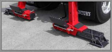
For even more stability in side pull situations, the rear outriggers are available with hydraulic extendable feet. The optional outriggers also include a flip down rear spade along with the flat pad that can be converted to a spade for side pulls.
