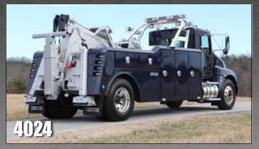
The 4024/T2 with over 103" of reach on the underlift is ideally suited to handle a wide variety of vehicles such as motor homes, delivery vans, and city tractors. This single axle unit with a 20-ton
