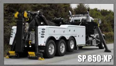
The SP 850-XP, available on the 7035 and 9055, combines the finest European technology with North America's most popular heavy-duty units. The hydraulic pivoting stiff legs and additional 35,000 lb. winches allow the operator much more power and flexibility in tough recovery situations including side pulls without shutting down roadways.
