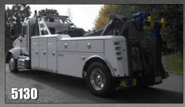
The 5130 is Century's Largest single axle integrated towing and ability to tow most vehicles without giving up maneuverability of and 25,000 lb. winches for your recovery and lifting applications.
