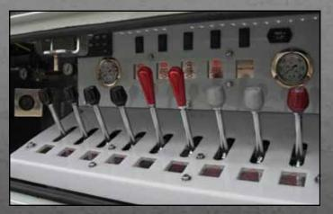
The Standard dual rear control stations provide smooth variable flow control of the functions at your fingertips. Dual pressure gauges, air winch clutch release switches, hour meter and air regulators are conveniently located in the polycarbonate control panel on driver side. Optional LED backlit control legends are available.
