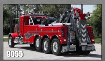
The 9055 is Century's largest capacity integrated towing and recovery unit. With a 50-ton recovery boom, with an optional third stage, and dual 50,000 lb. winches, the 9055 is ideal for heavy recovery work along with the ability to tow a wide variety of vehicles from mixers and packers through buses with its 138" of underlift reach.
