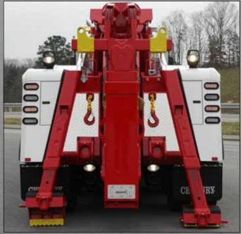
The diagonally opposed outriggers provide superior side and rear stability. The multi-position feet provide you with your choice of a flat pad or a spade with a replaceable grater blade. Optional "D" rings are available for low pull situations. An aluminum heel plate is also standard on the bottom side of the underlift to help protect your paint or lettering.
