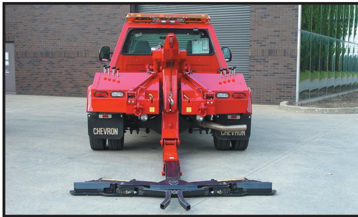
Chevron's optional AutoGrip II™ wheel lift allows the wheel retainer arms to hydraulically rotate from a fully closed storage position to a fully open approach position.
