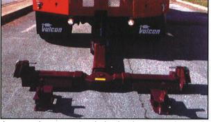
The 896 and 897 comes standard with Vulcan's patented 6,500 lb. strapless wheel retainer system. For heavier loads your underlift is equipped with a set of 3" low profile and 3" high profile lifting forks.
