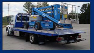
The 12 Series LCG™'s low-profile wheel lift stinger provides 66 inches of reach with a lift rating of 4,000 pounds. When retracted, the crossbar tucks in with minimal overhang. The LCG™ comes standard with the slide in L-Arm system, while the Vulcan strapless system and hydraulic Auto Grip systems are both optional.
