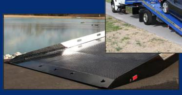
The SST® option is available on the 12 Series LCG<sup>†™</sup> steel carrier with removable blade rails and on the 12 Series aluminum carrier with solid, narrow-profile rails.
