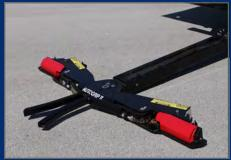
The Autogrip II self-loading wheel lift option operates from the control stations of the carrier by lowering the wheel lift, opening the claws and extending the crossbar until it comes into contact with the tires of the towed vehicle. The claws are then closed and the vehicle is ready to be lifted.
