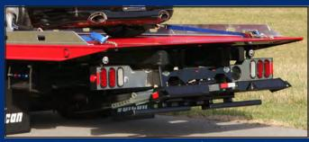
The LCG™ tailboard is equipped with easy access safety chains, an adjustable rear stabilizer and anti-theft L-arm storage.
