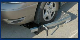
**Vulcan's Strapless Wheel** Retainer System is one of easiest and safest systems on the market today. The retainers pivot both vertically and horizontally for easy hook up in a variety of situations and best of all, no tie-down straps.
