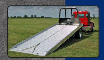
With a five- to six-inch lower deck height, the LCG™ allows for better stability and overhead clearance when hauling vehicles or equipment as well as increased operator safety because the operator can secure the equipment while standing on the ground. Additionally, the LCG™'s low load angle allows for easier loading overall.
