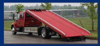
In addition to the low load angle, the LCG™ has a dump angle of 20°. This allows the operator to easily unload damaged vehicles or equipment.
