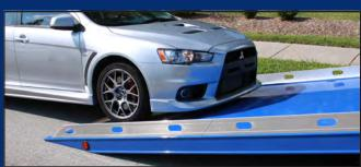
With a lower deck height and low load angle, the LCG™ allows the operator to load most vehicles without needing wood.
