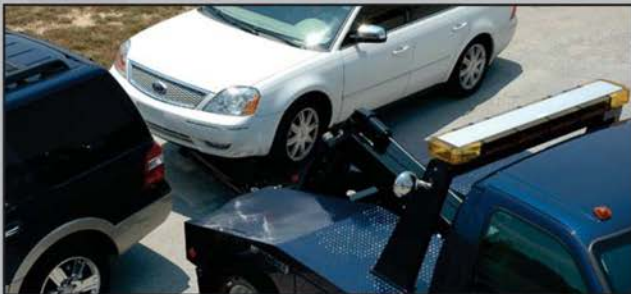
The Holmes 440-G2 is capable of hooking up to a vehicle at a 90° angle such as parallel parked vehicles.
