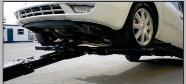
The Optional Power Tilt feature allows the wheel lift to operate through a 30-degree arc, which provides easier hook-ups on driveways or sloped roads.
