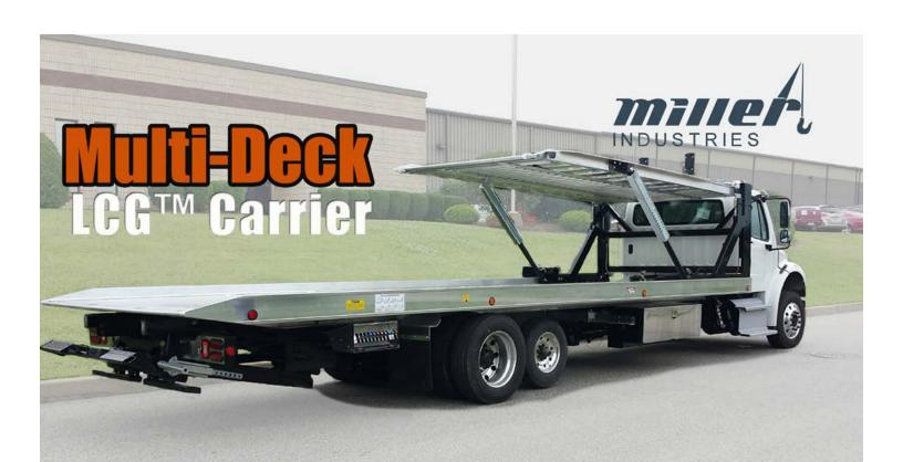
The combination of proven technology and reliability of a 16 Series Aluminum LCG™ (Low Center of Gravity) Carrier with an auxilary deck system. The Multi-Deck Carrier is available in deck lengths from 24-26 feet for hauling up to 3 vehicles as well as 30 foot decks for transporting up to 4 vehicles.
