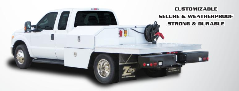
This MODULAR TRANSPORT unit features the same user-friendly storage compartments as the Modular Service Body along with a similar functional design, combined with many unique options. The powder coated aluminum front compartments offer a combined 32 cubic feet of accessible and secure storage. The ability to haul your equipment, big or small, is now made possible with the attachment of a gooseneck trailer or fifth wheel, plus an 80 gallon transfer tank.
