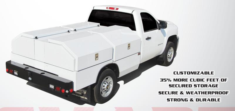
This MODULAR SERVICE model has unique, ergonomically designed, storage compartments with top lid openings to allow easy access and unobstructed visibility for its users. The low profile, powder coated aluminum, modular compartments offer up to 60 cubic feet of accessible, secure storage. The appealing body lines of this model, complete with its rugged, durable, and weatherproof design will protect your equipment against the elements, while keeping it organized, and easy to find.
