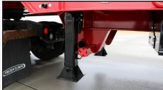
Jost 2-Speed Crank Down Landing Gear
