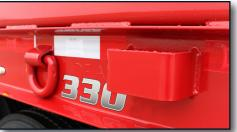
The standard four strap winches with opposing hooks and 4 "D" ring tie downs are conveniently located for efficiently securing the container.
