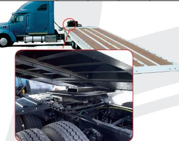
• Hinged Fifth Wheel Plate Extremely valuable when loading in tight places where the truck trailer is jackknifed. The fifth wheel plate will release and pivot before any stress is placed on your tractor fifth wheel.
