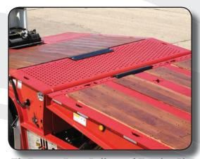
• Tie Downs, Front Roller, and Traction Plate Standard tiedowns are combination stake pocket "gotchas" for securement of equipment. The standard slope roller and steel wear plate act as a barrier against rubbing and prevent extra wear on the winch cable. The exclusive Landoll traction plate provides superior grip when loading onto the upper deck.
