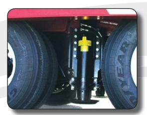
• Hydraulic Dock Levels Each leg is operated independently from the front control panel allowing the operator to raise 62,000 lbs. up to 54" high matching docks, platforms and other trailers.
