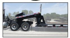
• 21<sup>1</sup>/<sub>2</sub>" Clearance, Cylinders Fully Extended (Temporary Clearance at Slow Speed)
