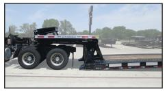
1½" Clearance with Teeth Seated in Fifth Tooth (4 Left, which will be needed with Front Flip Extension and One Axle Jeep Configuration)
