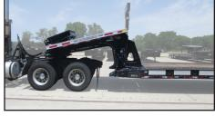
21½" Clearance, Cylinders Fully Extended (Temporary Clearance at Slow Speed)
