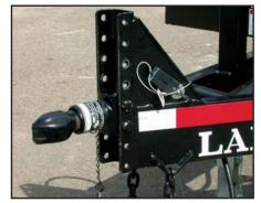
The hitch adjusts from 12" to 24" vertically.
