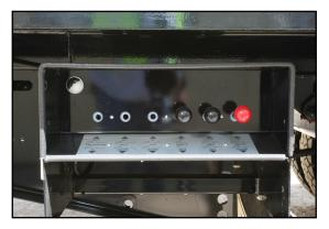
**Dual Hydraulic Controls** Well protected, illuminated hydraulic controls are located just rear of the axle.
