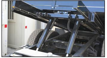
**Hydraulic System** The Loadoll II uses welded hydraulic cylinders with chrome plated rods for long trouble-free service.
