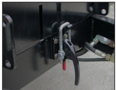
A heavy-duty bed lock-down with safety latch firmly secures the bed in transport position.
