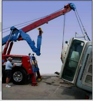
The SP 850-XP allows the operator to run the two winch cables from the XP unit to snatch blocks on the boom allowing a total of four winch lines.
