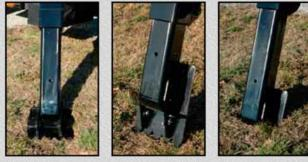
The swivel feet may be used as a flat pad for hard-packed surfaces or the operator may flip the plunger pin and lock the pad into a spade position for softer terrain applications.
