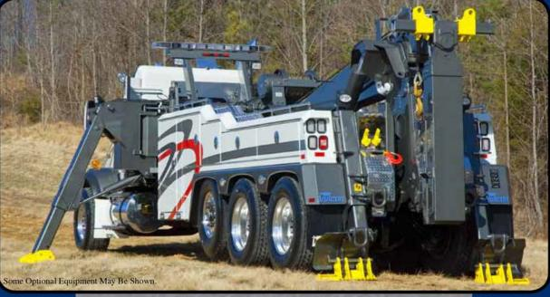
All recovery operators have experienced the problems of having traffic backed up with a casualty down in a ravine and the law enforcement not wanting to block lanes of traffic. The SP 850-XP option can solve these types of difficult situations with a pivoting hydraulic stiff-leg to handle tough side pull recoveries and eliminate the need to block more lanes of traffic than necessary.
