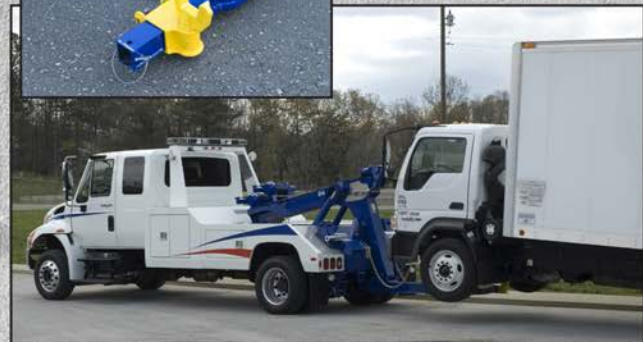
The fabricated underlift is rated at 7,000 lbs. lift capacity at its fully extended reach using lifting forks and has a tow capacity of 20,000 lbs. This makes the Vulcan V-24 ideal for towing a wide variety of light- and medium-duty trucks, as well as automobiles.
