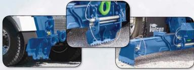
Independent rear spades provide a wide foot-print and are available with optional multi-position flipper feet or extendable rear outriggers.
