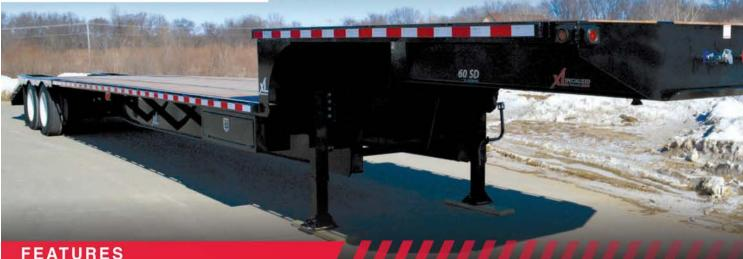
1 1/8-inch flush Apitong decking is stronger than Oak 3-inch channel crossmembers on 16-inch centers available with 48-foot or 53-foot overall length built to last, using T-1 flange and 80K webs 3/8" x 2" rub rail with single pipe spools stake pockets on 24" centers knee braces on 48" centers mill channel side rails
