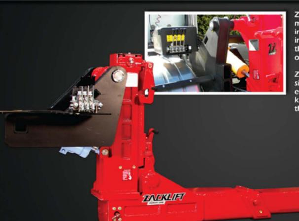
Zacklift has spent 30 years engineering the permanent mounting. All heights and angles have been engineered into the single piece of mounting hardware that is utilized in the installation. Every step of the process is guided, as this pre-engineered framework is permanently mounted over the truck frame.
