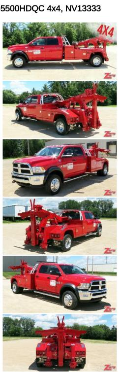
TM22G - 22" Wireless Tow Light 408-512TA-HRS - Hydraulic Rear Spades SVLCD50-29-620 - Rear Vision Camera System PW Complete w/Boom - Painting Complete MR6FM-A - Qty. 2, Amber Strobes Mounted On Tailboard
