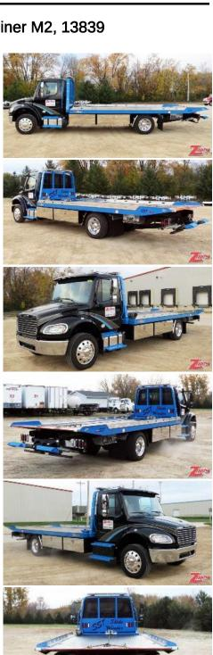
1 Set J-Chains Straps/Rachets Dual Controls Rear Safety Chains CR6 Plug In Hook Up Lights Wheel Lift L-Arms Stainless Steel Quarter Fenders Extra Lights On Pylon, Bed Sides & Tailboard 102" Wide Tow Light Kit
