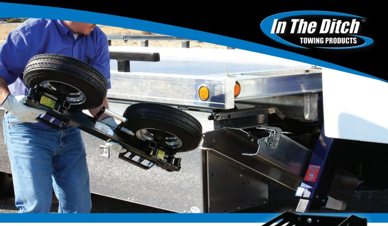
The ITD1347 Car Carrier Dolly Mount makes storing your Speed® Dolly on a car carrier easy. The steel portion mounts to your truck frame, while the aluminum portion holds a single Speed® Dolly. Features an integrated lock system that can be pad-locked. Can be adjusted to fit all 4:80 x 8 tires.
