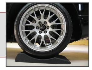
FlatStoppers were developed as a solution for people having problems with tires developing flat spots when a vehicle is parked for 30 days or longer. Once tires are set on FlatStoppers (on a level surface), they settle into the ramps concave depression, which helps support more of the tire. This disperses the weight of the car more evenly onto the tire, helping to prevent any flat spotting.
