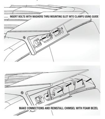
**7. Final Securing of the Platform:** BE SURE TO CENTER AND LEVEL THE PLATFORM ON THE VEHICLE CAB. Holding the Platform Assembly firmly against the vehicle, tighten the clamp adjustment fasteners to take up the slack until the gaskets fit uniformly against the profile of the cab body and compress the leading edge deflector gasket. Sight the top of the endcaps as a reference for level and true. Final tighten both clamp fasteners equally, 15-18 ft/lbs each.
