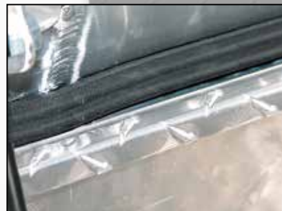
Full weather stripping keeps dust and moisture out.
