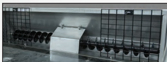
6" dia. auger and screen
