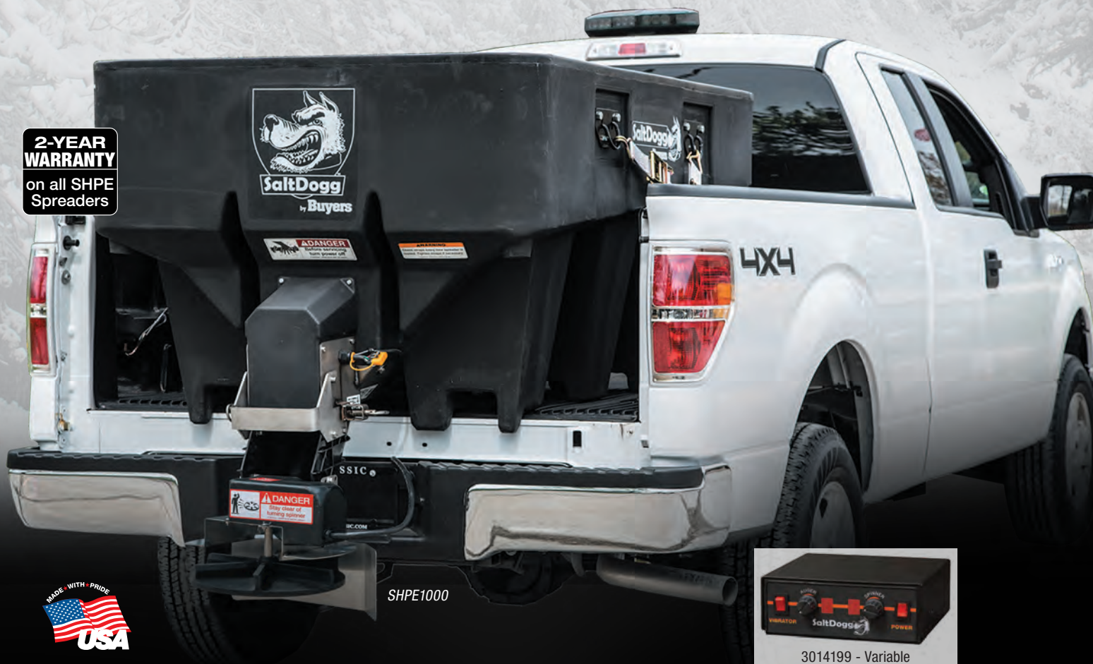
Features high flow chute with larger 14" spinner, open trough, and NEW stainless steel spinner shield
