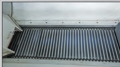
30.25" wide conveyor with 1/2" bars
