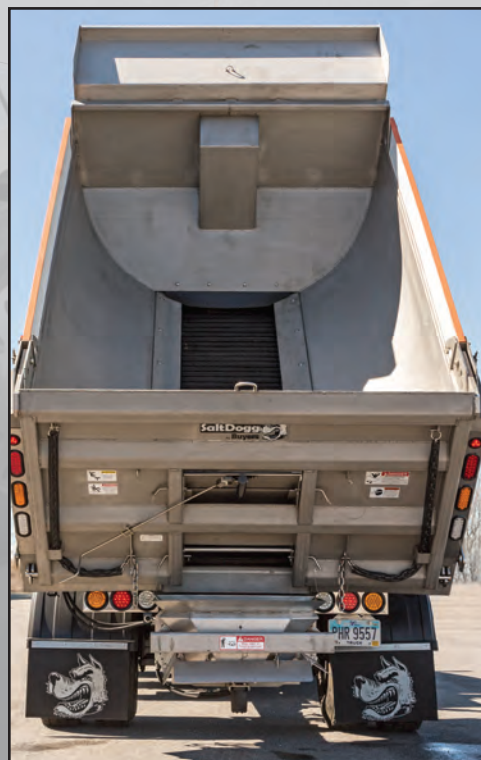
Unique, roll-formed sides and cross memberless floor design
