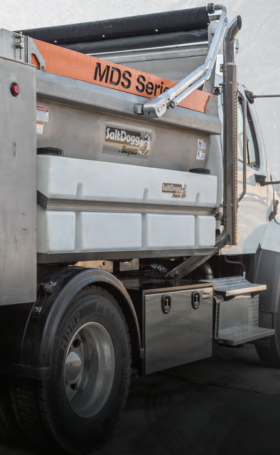
Unique, roll-formed sides and cross memberless floor design
