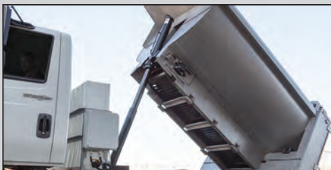
Mailhot® multi-stage, double-acting, nitrided cylinder, trunnion-mounted hoist
