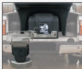
Swing-away chute for bulk unloading
