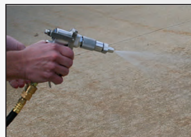
Adjustable spray nozzle - pressure switch activates pump on demand
