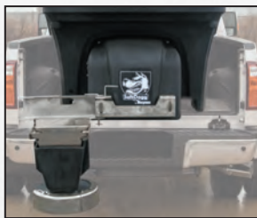
Swing-away chute for bulk unloading
