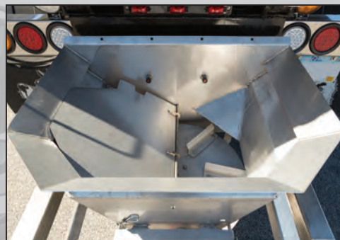
"Hex flow" chute and 24" spinner with adjustable baffles for optimal spread pattern
