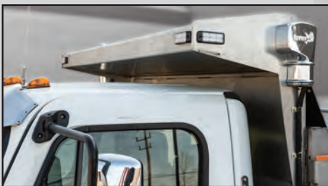
Cab shield with Built-In Tarp System
