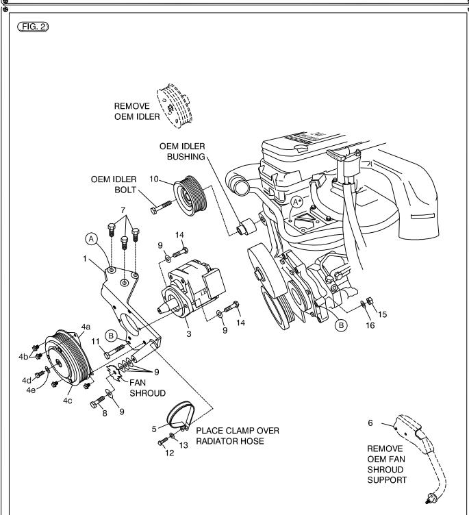
\*The three mounting bolts at Location A must be clear of factory mounted options and modules.
