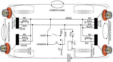
The front and rear heads are configured to flash independently of each other. In order to have the front and rear heads flash in sychronization, the blue wires from all units must be connected. The yellow wire can then be used to determine either alternate or simultaneous flash between each unit in the system by connecting to either power or ground.
