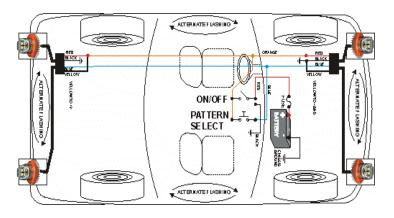
For ease of installation, all dual head products incorporate a connector between the LED head and power module. This will allow you to route the wires from each head individually to the power module eliminating the need to drill large pass thru holes. If installed in a wet area the connections can be sealed with RTV as shown below.
