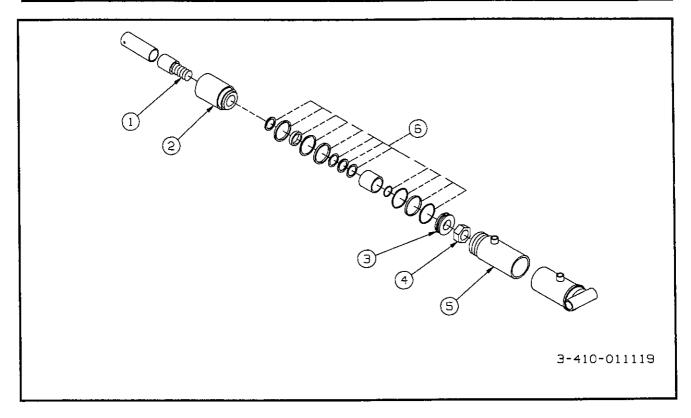
Figure 8-9 Trailer Tilt Cylinder
