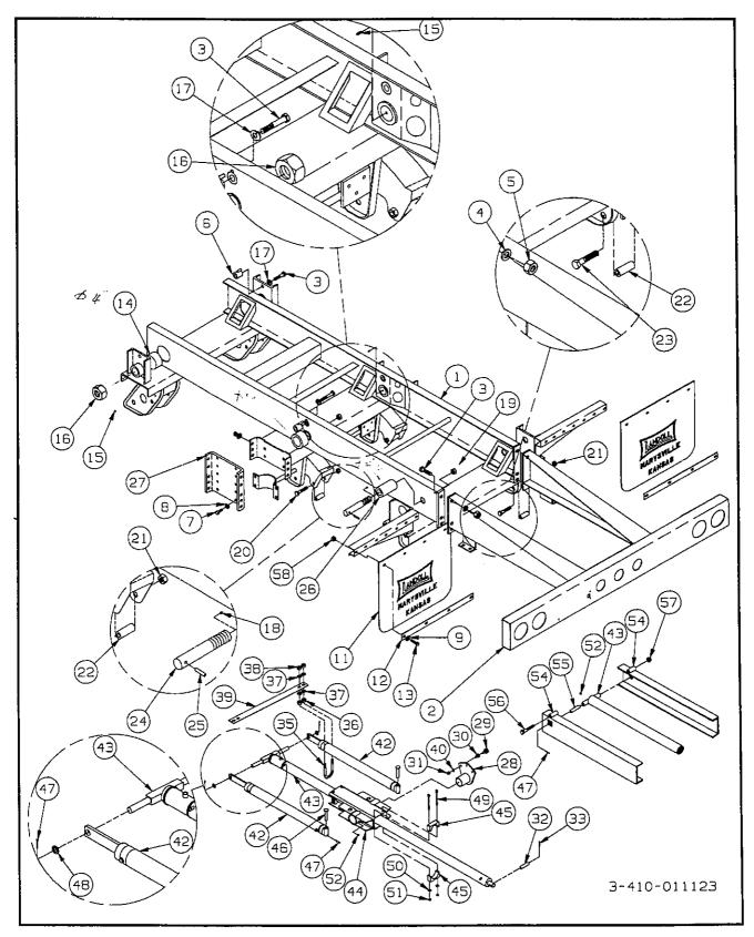
Figure 8-11 Spring Suspension Undercarriage
