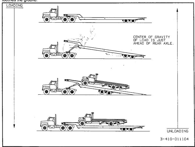
Figure 5-2 Steps for Loading & Unloading
