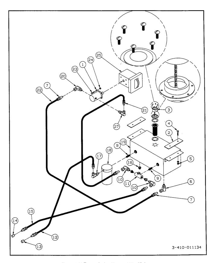
Figure 8-30 Transmission Mounted Wet Kit Items
