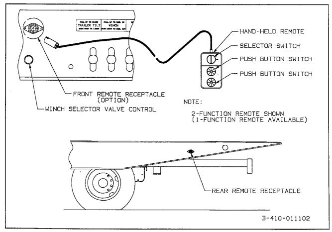
Figure 4-7 Electric Remote Controls
