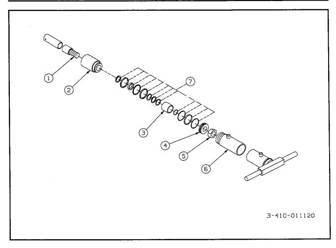
Fig. 8-10 Undercarriage Slide Cylinder (Low Load Angle)
