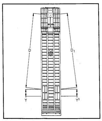
Figure 6-9 Checking Axle Alignment
