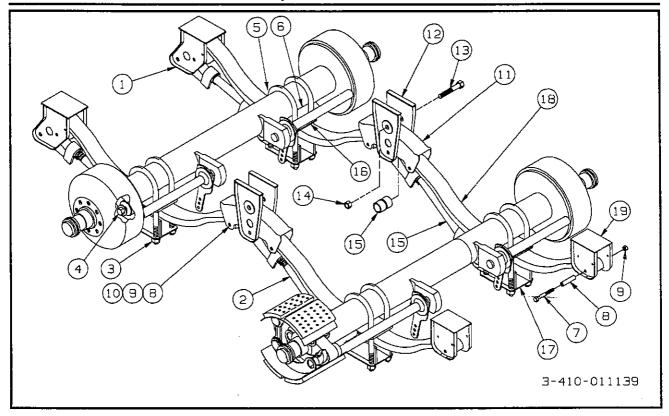
Figure 8-18 Single Leaf Spring Suspension
