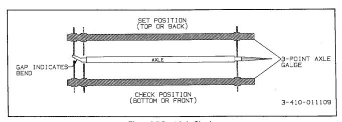
Figure 6-7 Bent Axle Check
