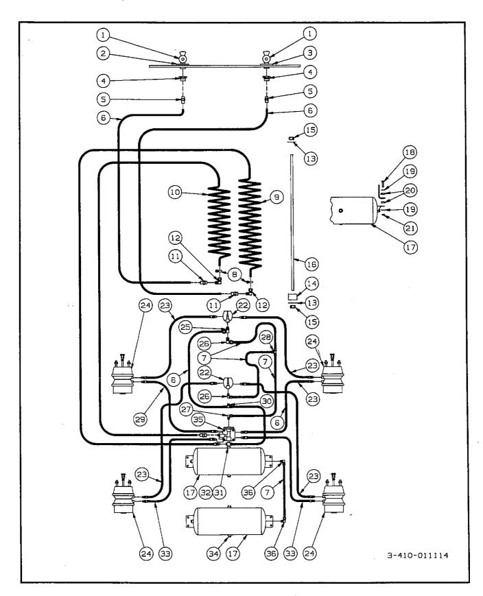
Figure 8-3 Tandem Spring Brake Schematic
