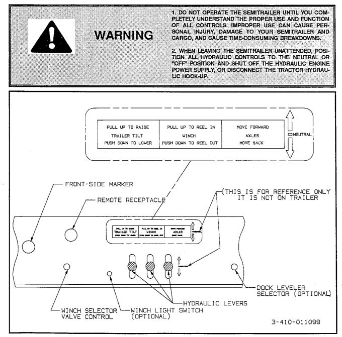
Figure 4-1 Hydraulic Control Levers
