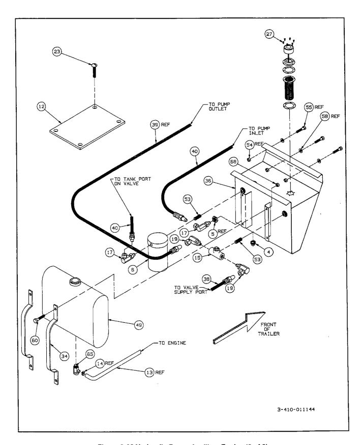
Figure 8-29 Hydraulic Power Auxiliary Engine (2 of 2)
