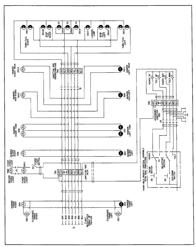
Figure 6-11 - 317A Wiring Diagram
