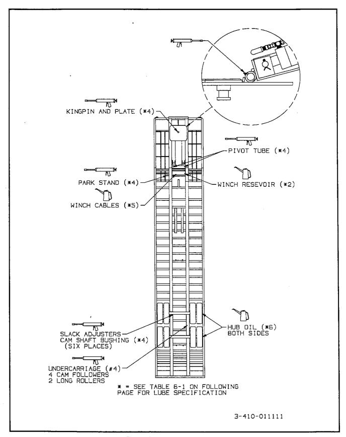
Figure 6-10 Lubrication Points
