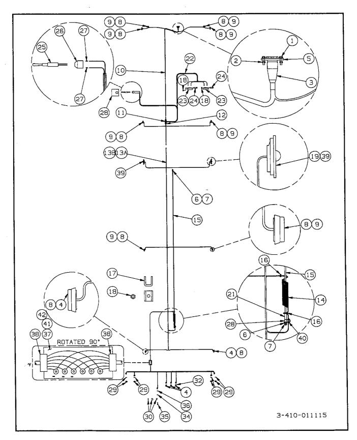
Figure 8-4 - 317 Electric System Schematic
