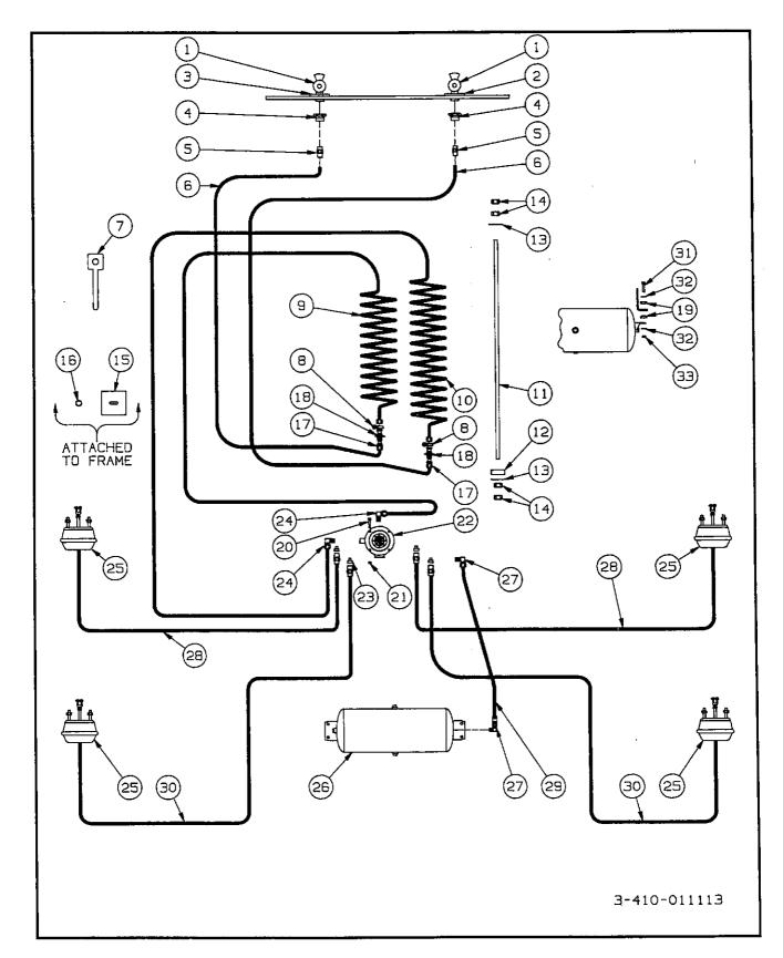
Figure 8-2 Tandem Air Brake Schematic
