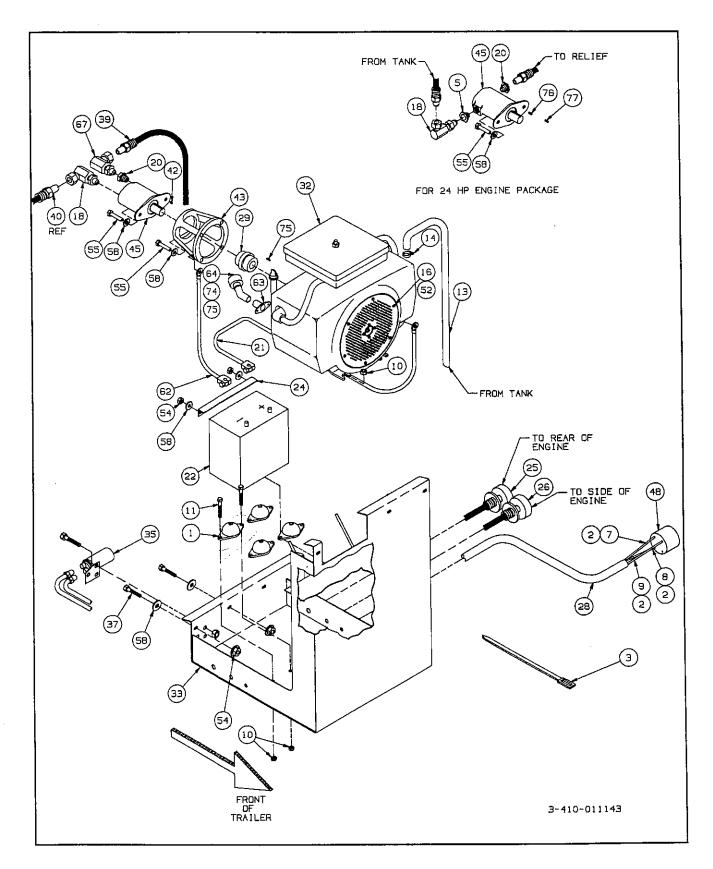
Figure 8-28 Hydraulic Power Auxiliary Engine (1 of 2)
