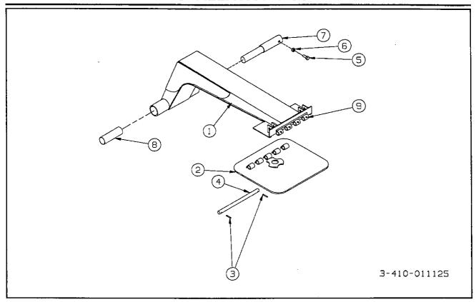
Figure 8-14 Hitch Installation Assembly Parts
