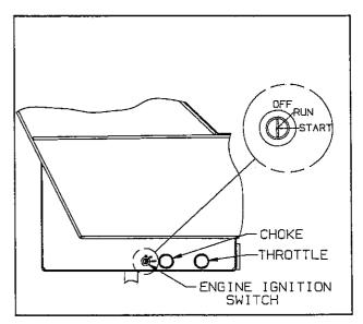
Figure 4-5 Engine Ignition Switch
