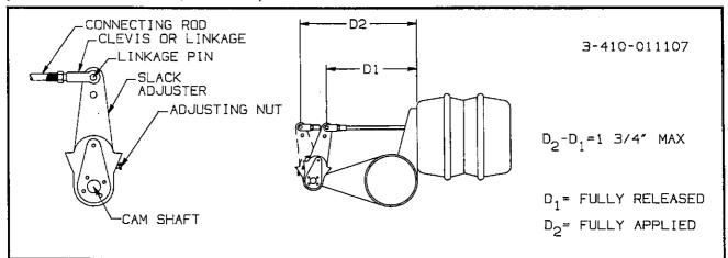
Figure 6-2 Checking Brake Adjustment
