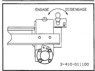
Figure 4-4 20,000# Winch Clutch
