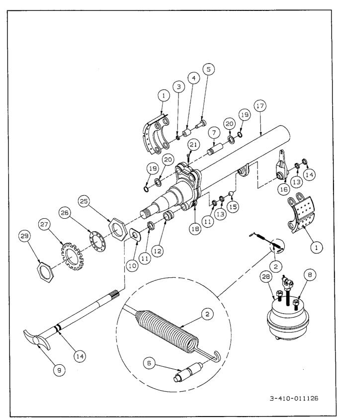
Figure 8-16 Semitrailer Axle Parts
