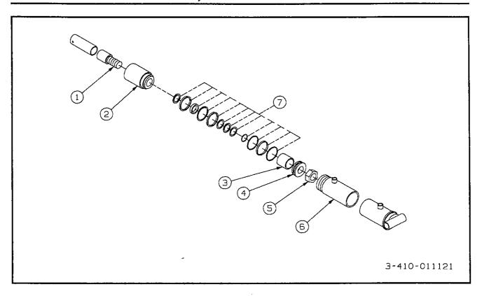
Figure 8-7 Low Load Angle Cylinder
