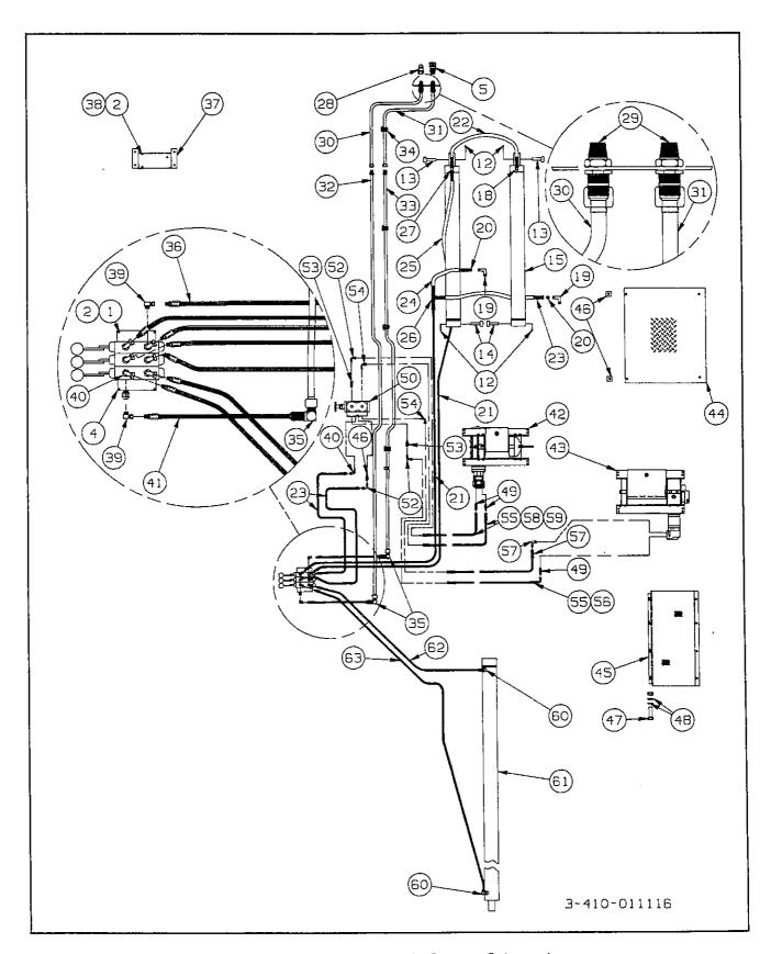
Figure 8-5 Standard Hydraulic System Schematic
