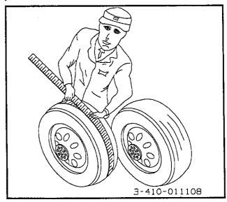
Figure 6-4 Checking Tire Size with Measuring Tape
