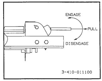
Figure 4-3 12,000# Winch Clutch
