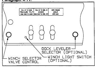
Figure 4-2 Winch Selector Valve Control
