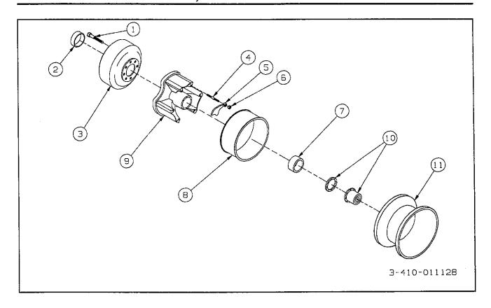
Figure 8-17 Three Spoke Hub & Drum Items
