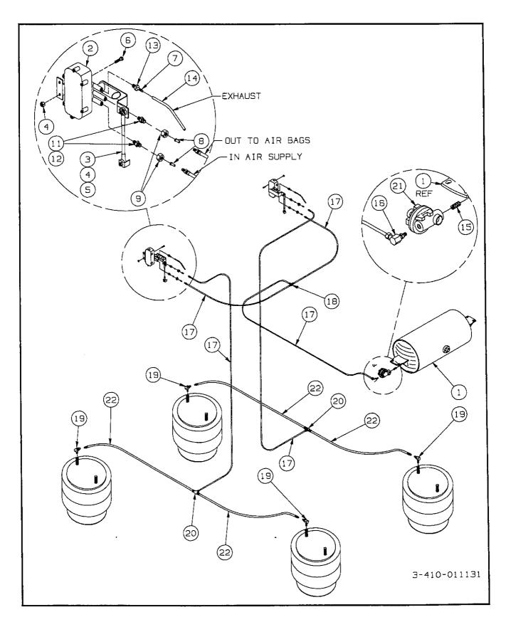
Figure 8-20 Tandem Air Suspension Plumbing
