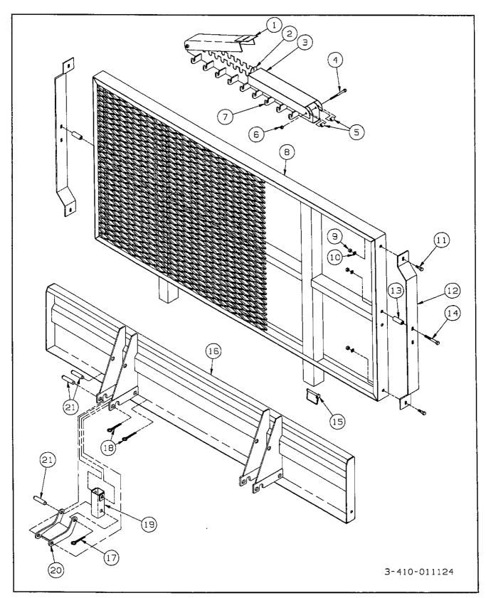
Figure 8-13 Front Extension & Bulkhead items
