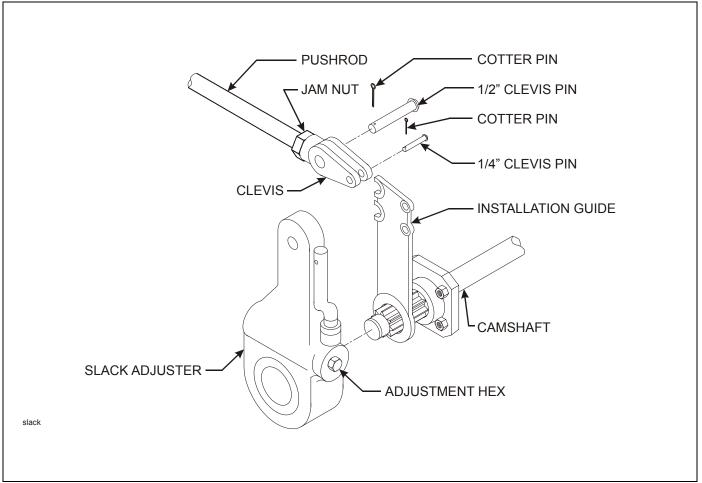
Figure 4-11: Automatic Slack Adjuster
