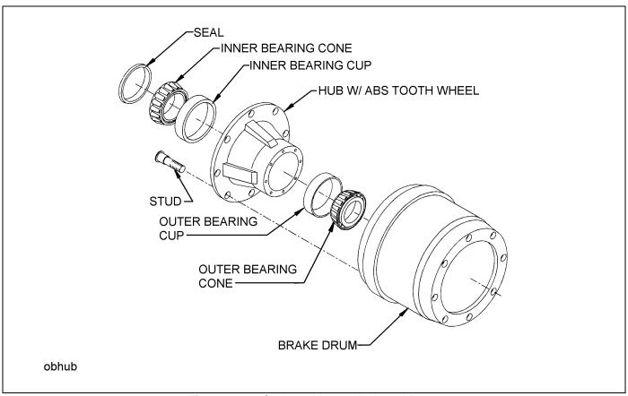
Figure 4-12: Outboard Mount Hub and Drum
