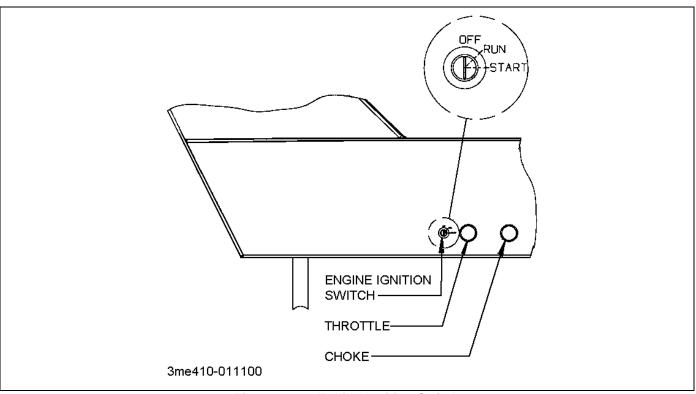
Figure 3-12: Engine Ignition Switch
