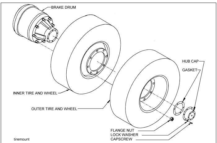
Figure 4-16: Mounting Tires and Wheels
