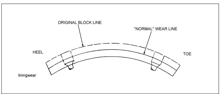
Figure 4-10: Brake Lining Wear
