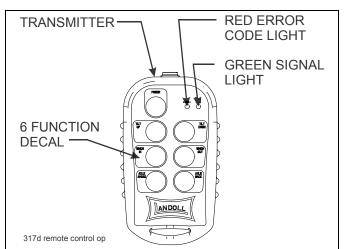
Figure 3-10: Remote Control Transmitter
