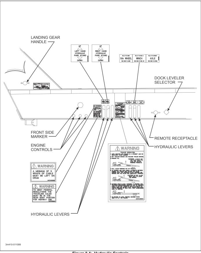
Figure 3-4: Hydraulic Controls
