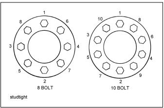
Figure 4-17: Stud Tightening Sequence
