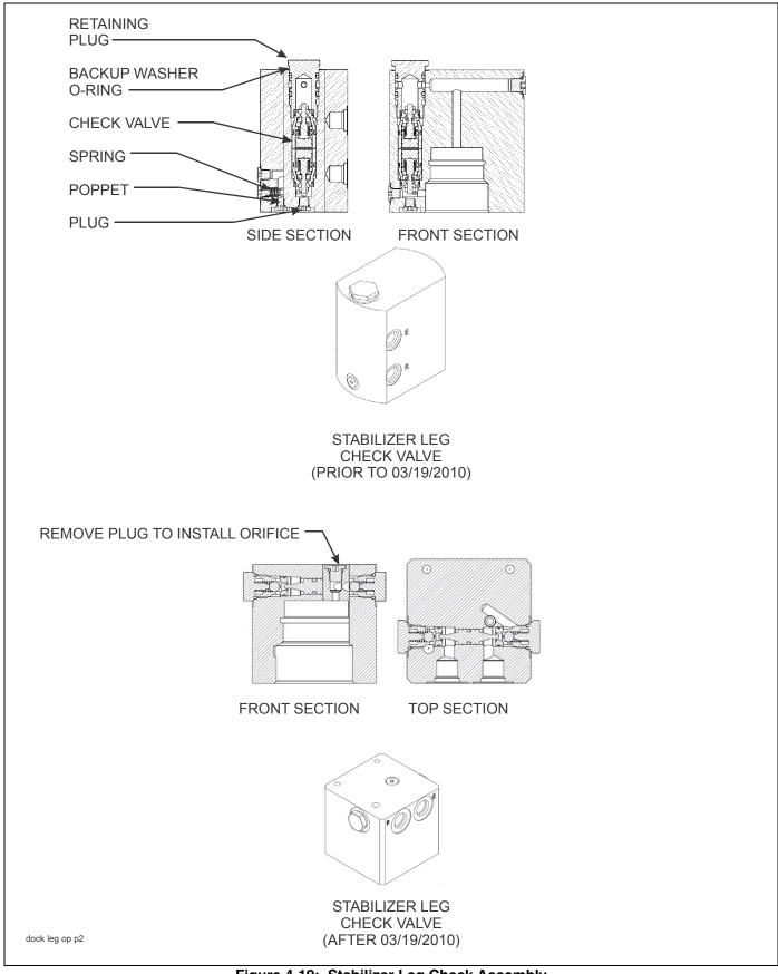
Figure 4-19: Stabilizer Leg Check Assembly
