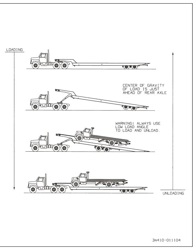
FIGURE 3-6 STEPS FOR LOADING AND UNLOADING
