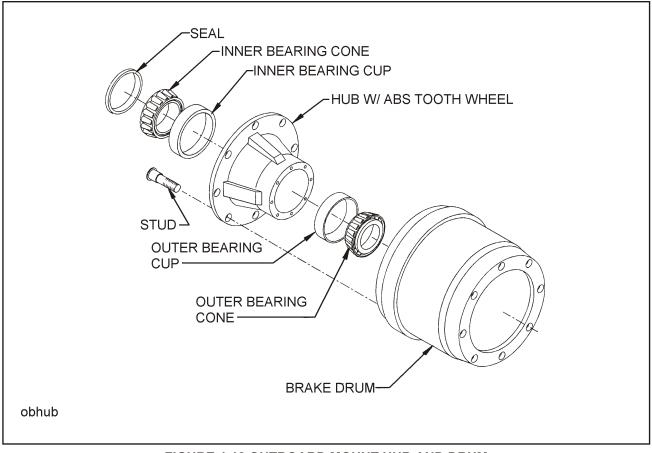
FIGURE 4-12 OUTBOARD MOUNT HUB AND DRUM
