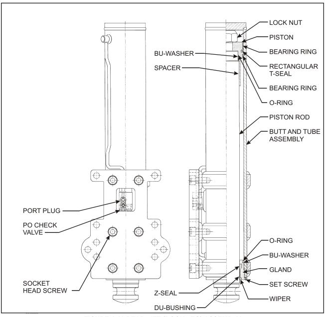
FIGURE 4-18 REAR LIFT (DOCK LEG) ASSEMBLY
