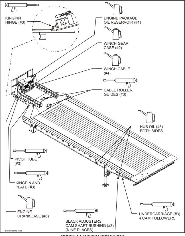
FIGURE 4-1 LUBRICATION POINTS
