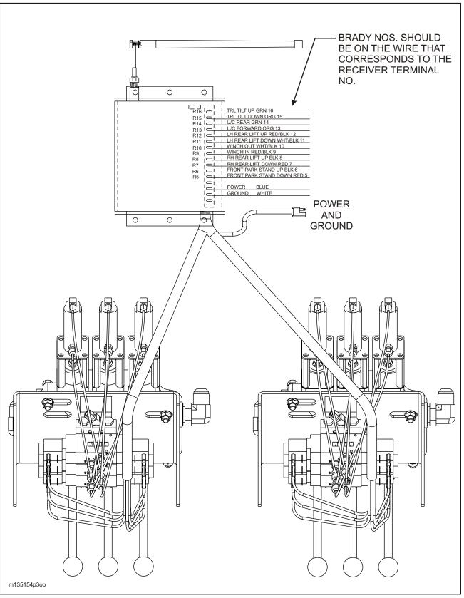
FIGURE 4-3 REMOTE WIRING DIAGRAM
