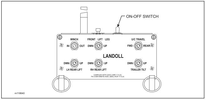
FIGURE 3-4 REMOTE CONTROL SWITCH PANEL
