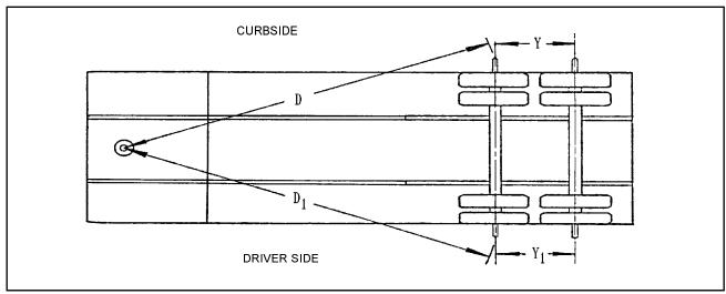
Figure 4-8 Checking Axle Alignment
