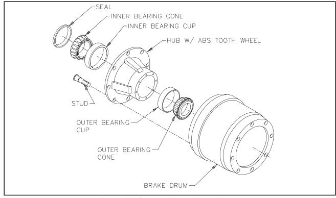
Figure 4-14 Outboard Mount Hub and Drum
