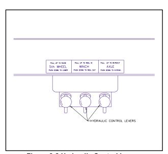
Figure 3-2 Hydraulic Control Levers
