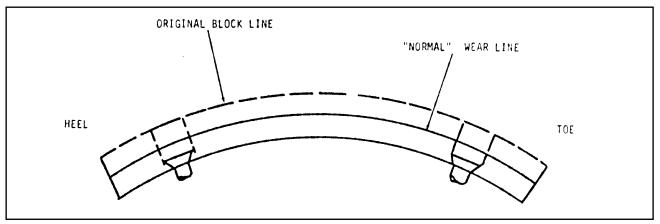
Figure 4-10 Brake Lining Wear
