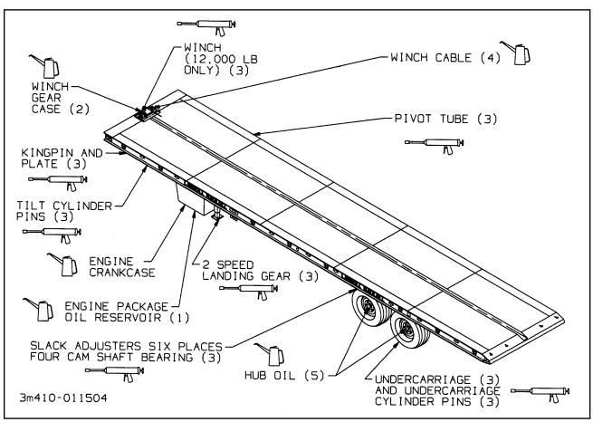
**Figure 4-1 Lubrication Points**
