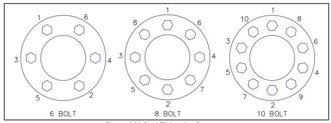
Figure 4-20 Stud Tightening Sequence
