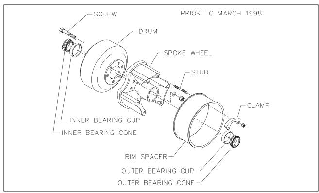
Figure 4-13 Three Spoke Wheel and Drum
