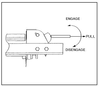
Figure 3-4 12,000# Winch Clutch
