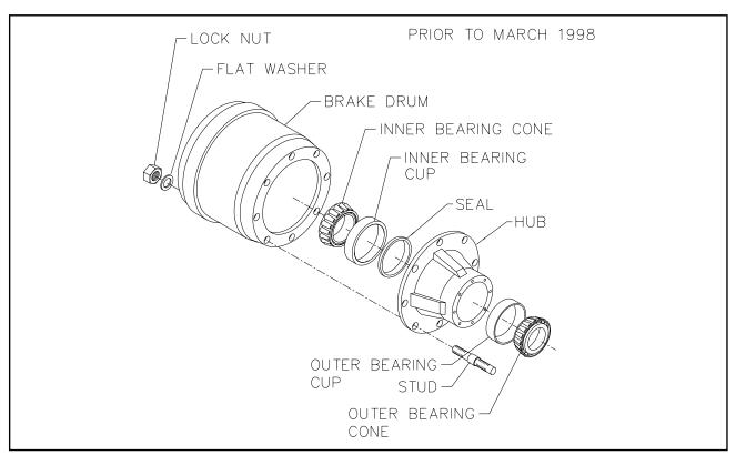
Figure 4-15 Inboard Mount Hub and Drum
