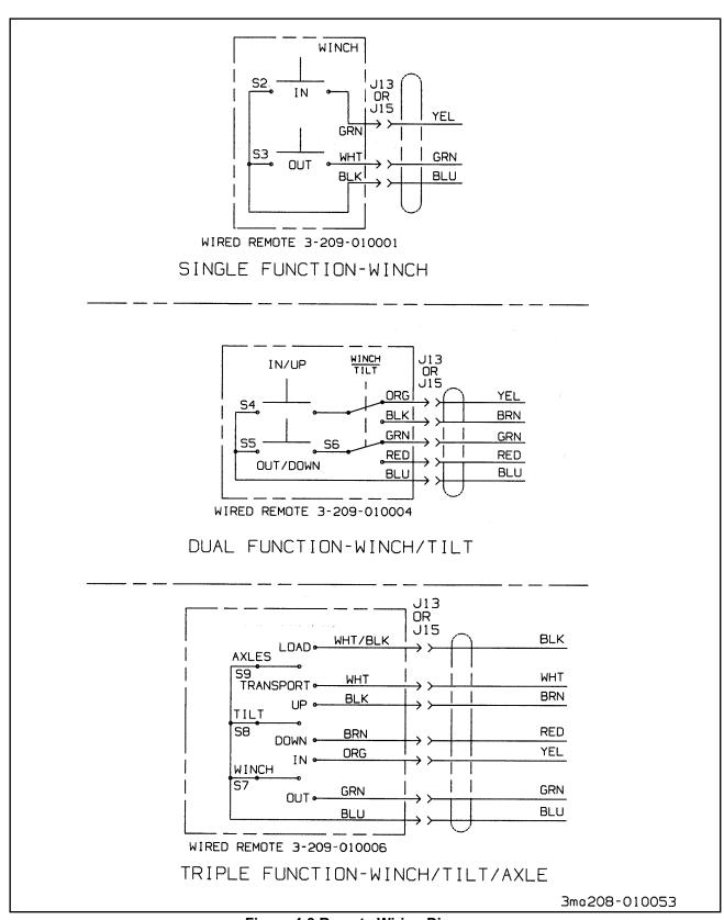
Figure 4-3 Remote Wiring Diagram
