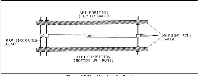
Figure 4-7 Checking Axle for Bend
