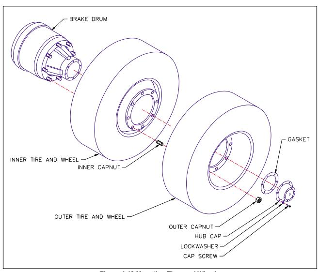
Figure 4-19 Mounting Tires and Wheels
