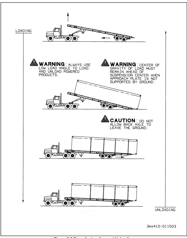
Figure 3-3 Steps for Loading and Unloading
