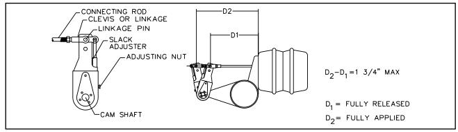
Figure 4-12 Checking Brake Adjustment
