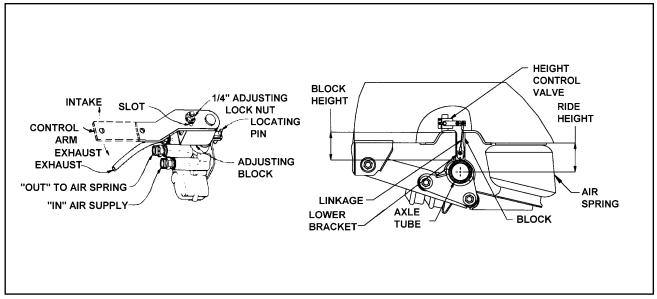
Figure 4-5 Air Ride Height Adjustment
