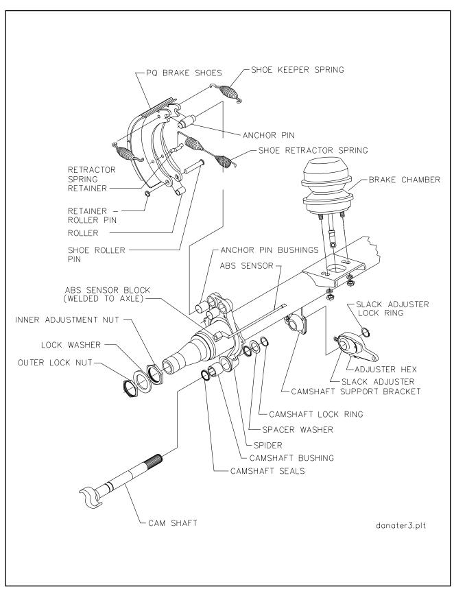
Figure 4-11 Axle and Brake Assembly
