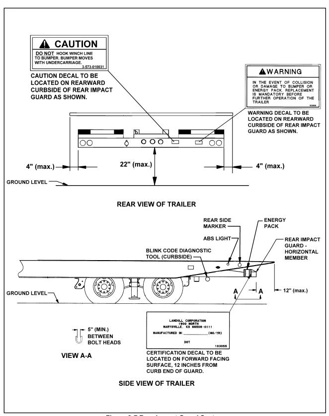
Figure 3-7 Rear Impact Guard System
