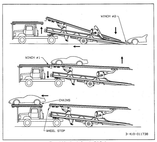
Figure 3-8 Loading the Over-the-Cab Deck
