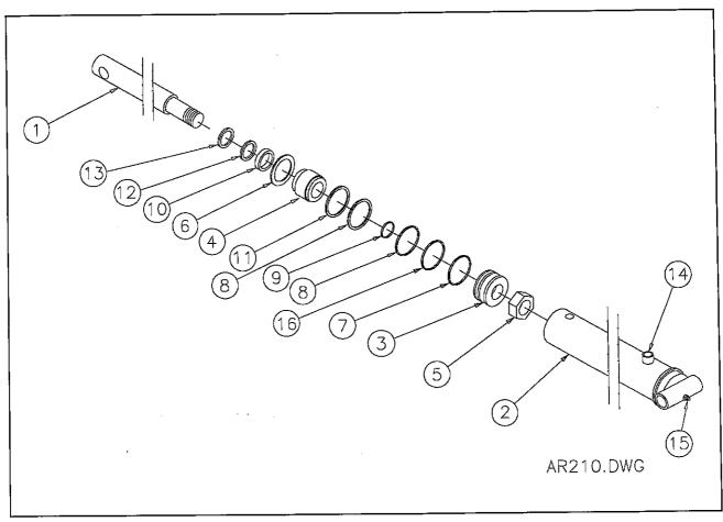
Figure 6-12 Hydraulic Cylinder Assembly, 4"x36"
