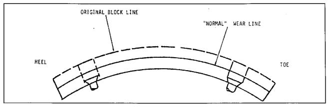
Figure 4-9 Brake Lining Wear
