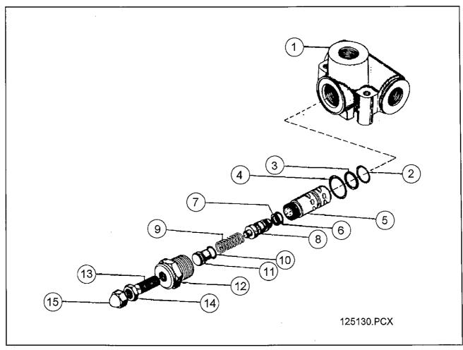
Figure 6-43 Pressure Relief Valve
