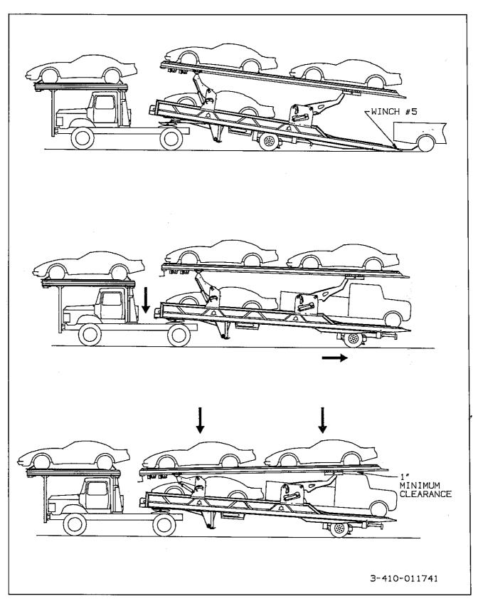
Figure 3-11 Loading the Lower Deck
