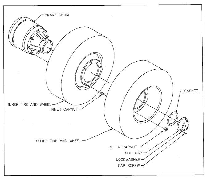
Figure 4-19 Mounting Tires and Wheels
