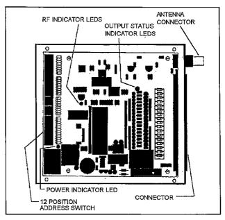
Figure 4-3 Receiver Printed Circuit Board .
