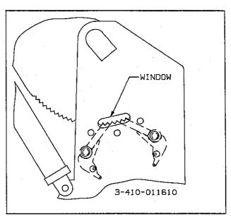
Figure 3-5 Lock Verification Window
