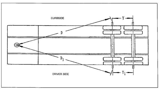
Figure 4-7 Checking Axle Alignment
