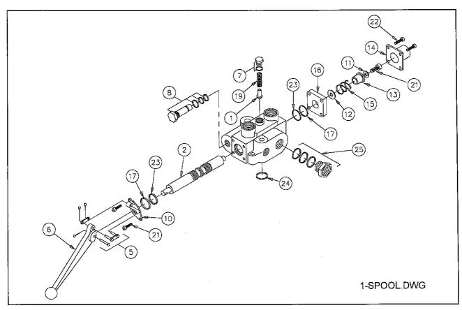
Figure 6-39 Hydraulic Single Spool Valve
