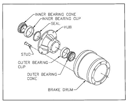
Figure 4-14 Outboard Mount Hub and Drum
