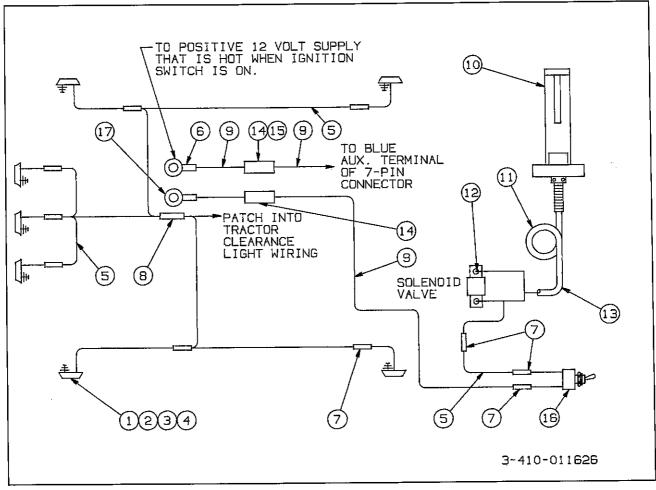
Figure 6-35 "Over-the-cab" Electrical Assembly
