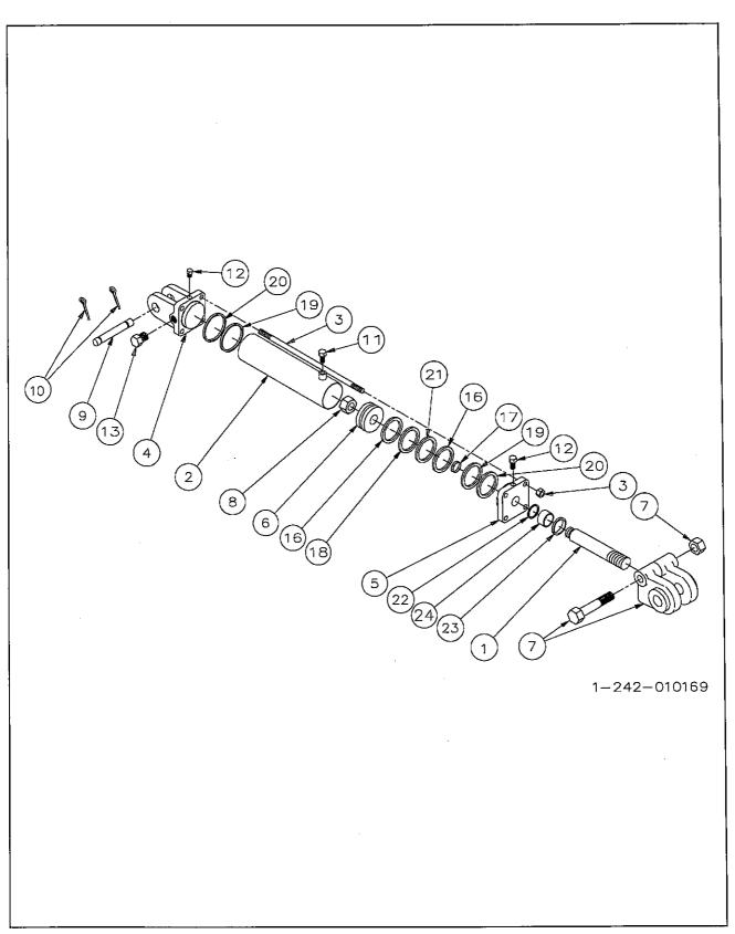
Figure 6-11 Hydraulic Cylinder Assembly, 16" Upper Deck Lift Cylinders (See Fig. 6-9 for location)
