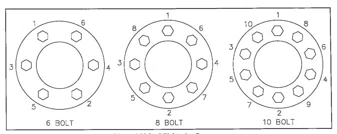
Figure 4-20 Stud Tightening Sequence
