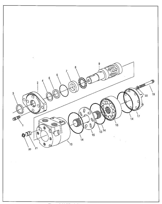
Figure 6-28 Winch Motor Assembly 8,000#
