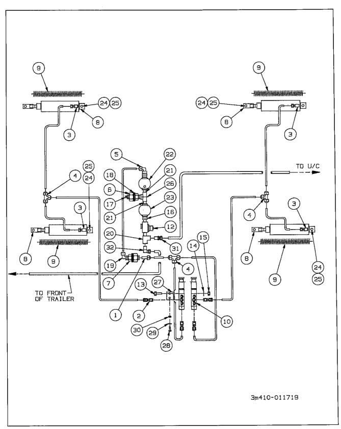
Figure 6-5 Deck Lock Air System
