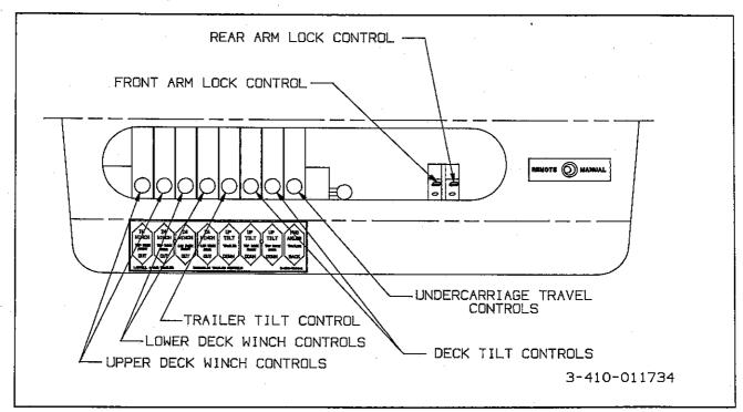
Figure 3-2 Hydraulic Control Levers
