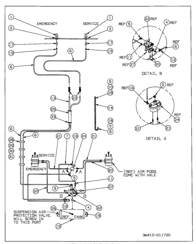
Figure 6-23 Air Brake System
