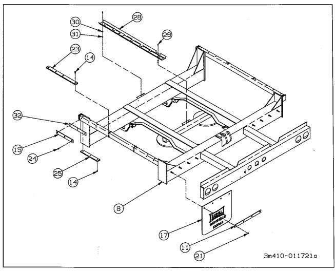
Figure 6-19 Undercarriage Assembly
