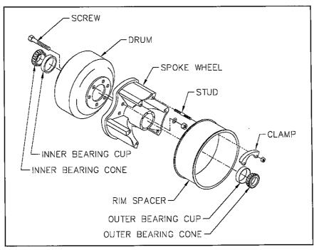
Figure 4-13 Three Spoke Wheel and Drum
