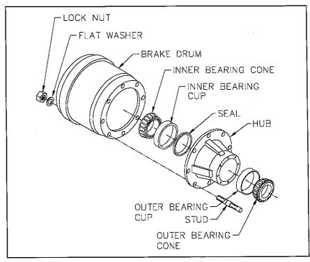
Figure 4-15 Inboard Mount Hub and Drum
