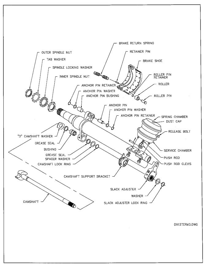
Figure 4-10 Axle and Brake Assembly
