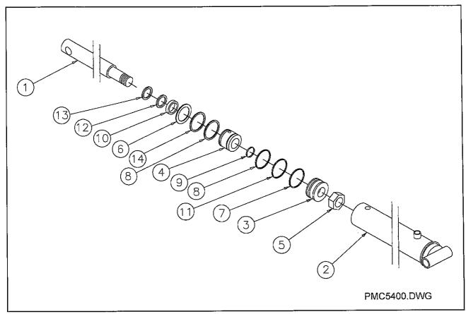
Figure 6-37 Hydraulic Cylinder 3" X 48"
