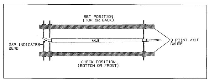
Figure 4-5 Checking Axle for Bend
