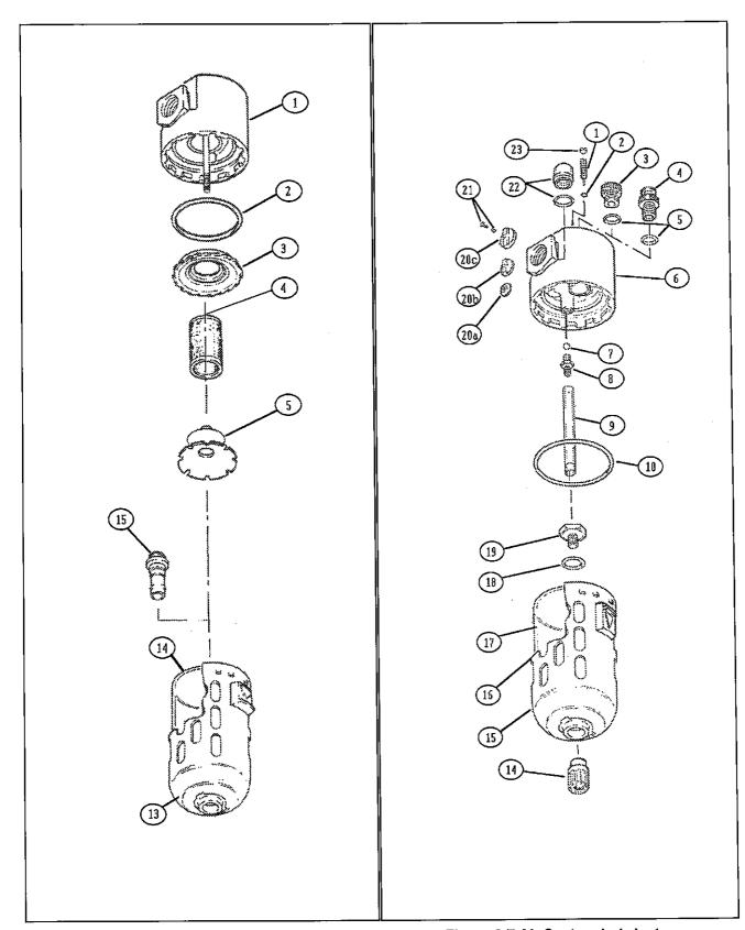
Figure 6-6 Air System Filter
