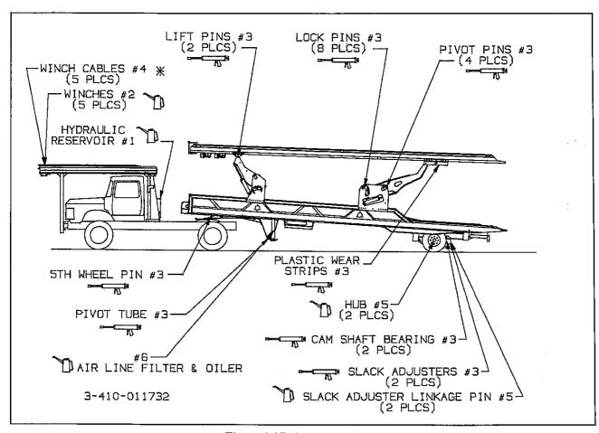
Figure 4-1 Lubrication Points
