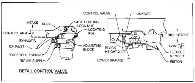
Figure 4-4 Air Ride Height Adjustment
