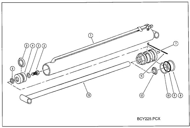
Figure 6-38 Hydraulic Cylinder 2-1/2" X 32"
