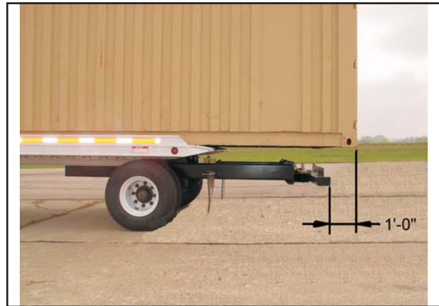
Figure 3-10 Distance Between U/C and Container
