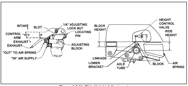
Figure 4-3 Air Ride Height Adjustment
