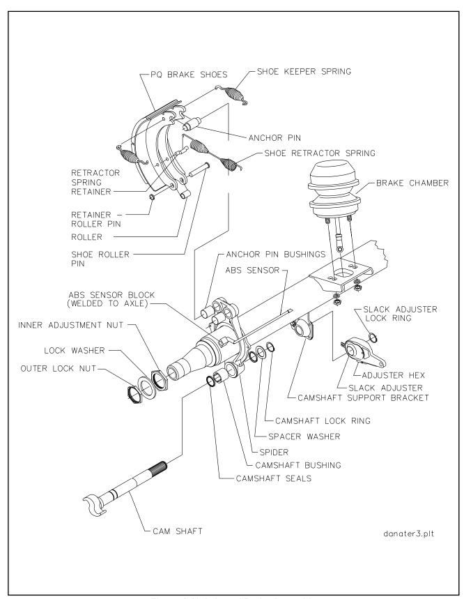
Figure 4-10 Axle and Brake Assembly
