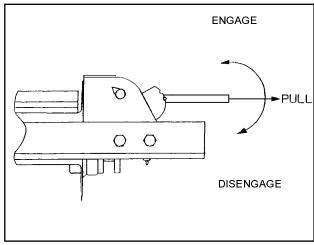
Figure 3-3 12,000# Winch Clutch
