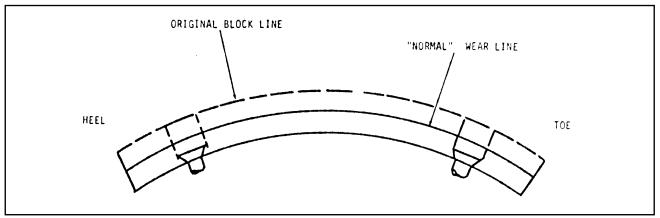
Figure 4-9 Brake Lining Wear
