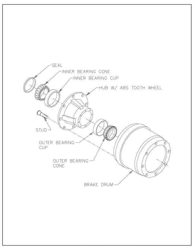
Figure 4-12 Outboard Mount Hub and Drum
