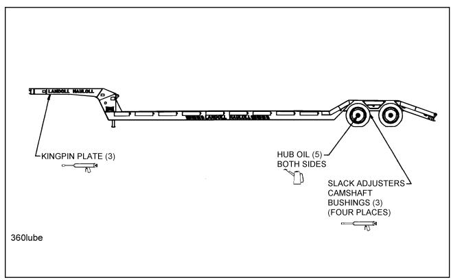
Figure 4-1 Lubrication Points
