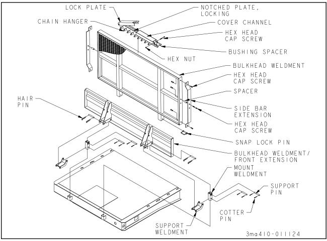
Figure 3-5 Front Extension/Bulkhead
