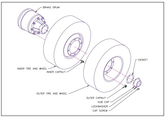
Figure 4-16 Mounting Tires and Wheels
