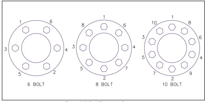
Figure 4-17 Stud Tightening Sequence
