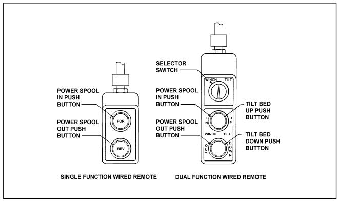
Figure 3-6 Examples of Remote Control Options
