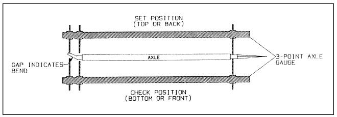
Figure 4-5 Checking Axle for Bend
