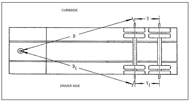
Figure 4-6 Checking Axle Alignment
