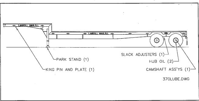
Fig. 4-15 Lubrication Points
