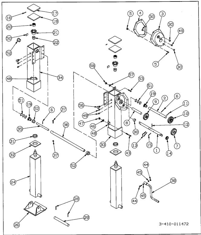
Fig. 4-14 Crank Landing Gear Assembly
