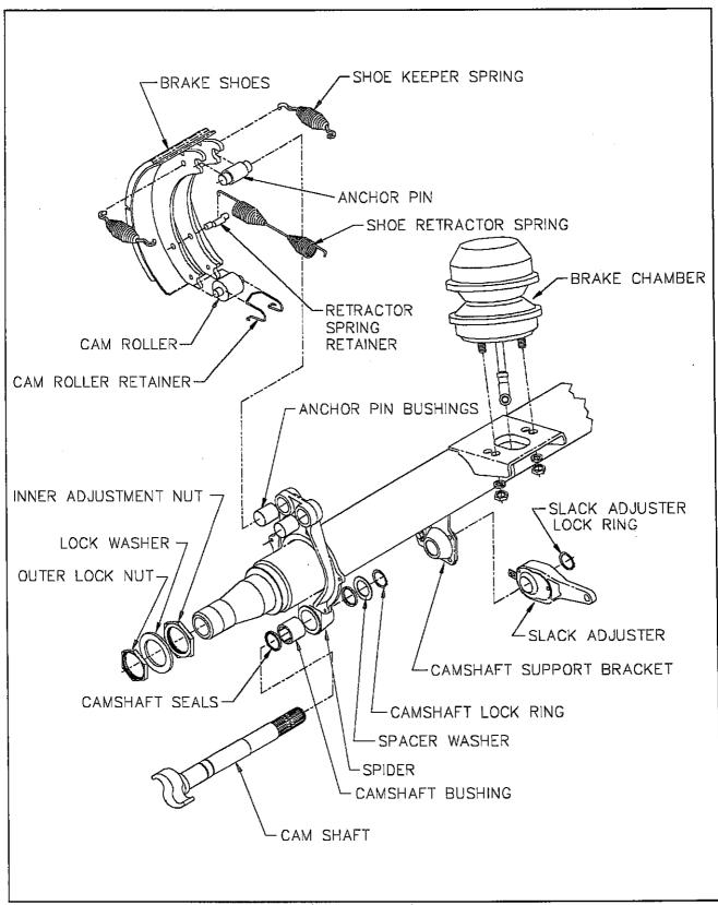
Fig. 4-3 Axle and Brake Assembly
