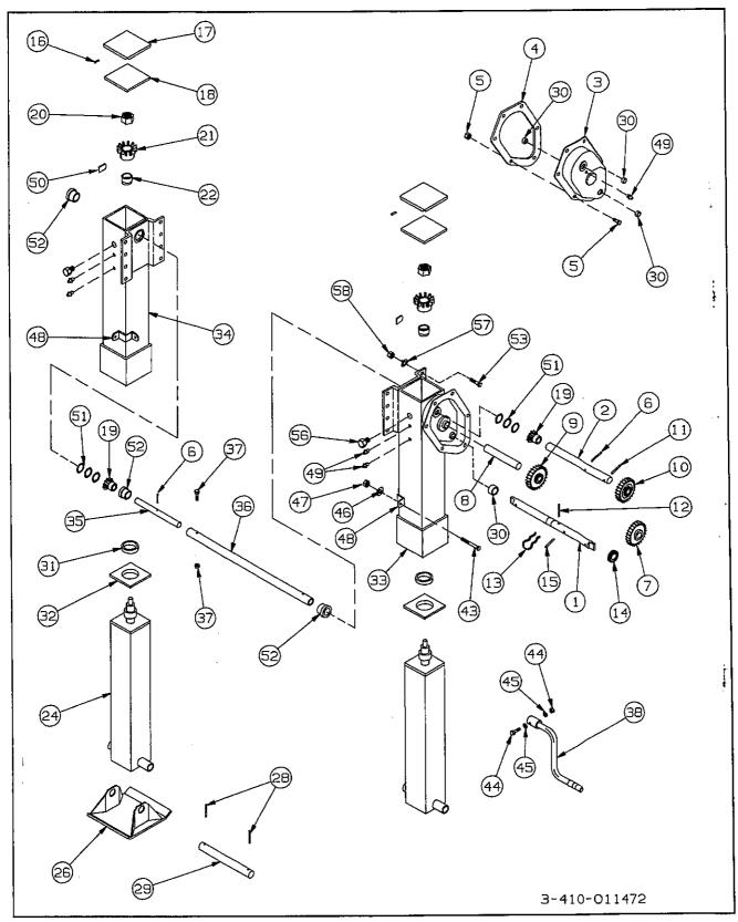
Figure 6-13 Crank Landing Gear Assembly
