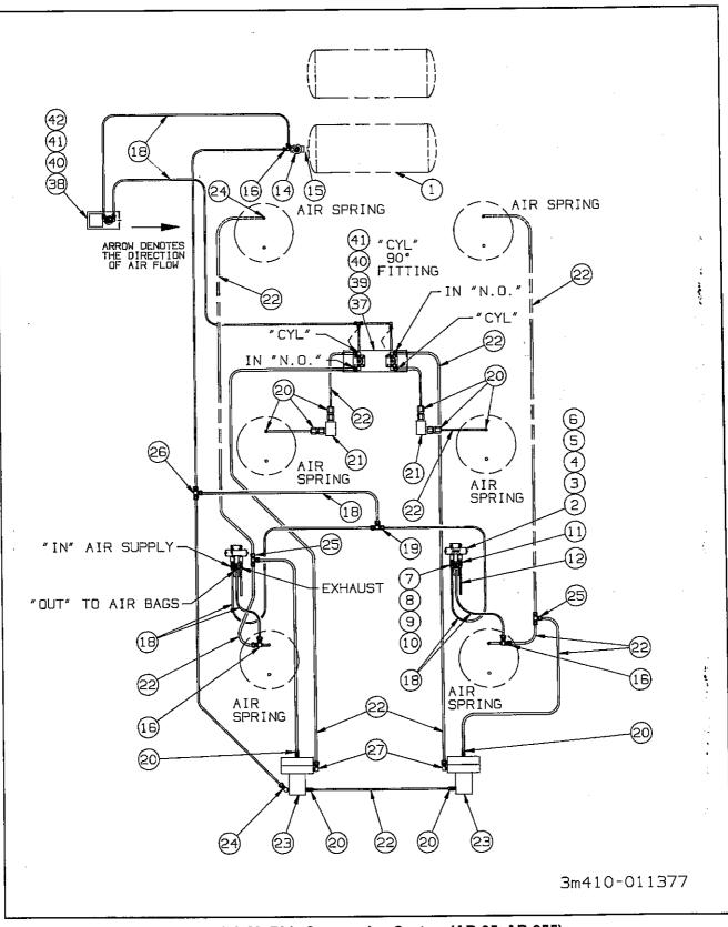
Figure 6-8 Air Ride Suspension System (AR-95, AR-955) Center Lift Axle
