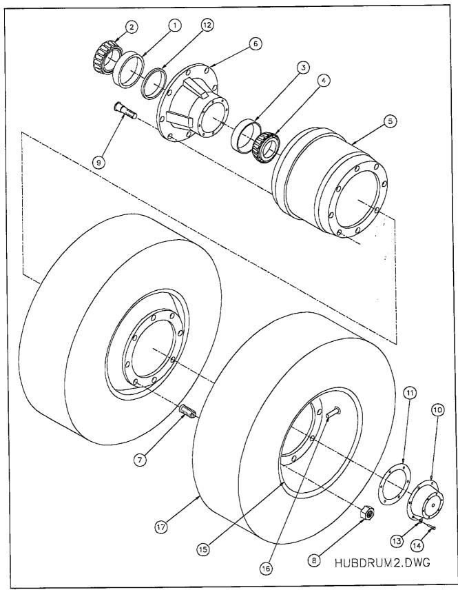
Figure 6-15 Outboard Hub and Drum Assembly
