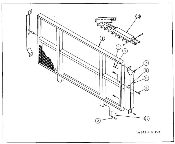
Figure 6-11 Bulkhead Assembly
