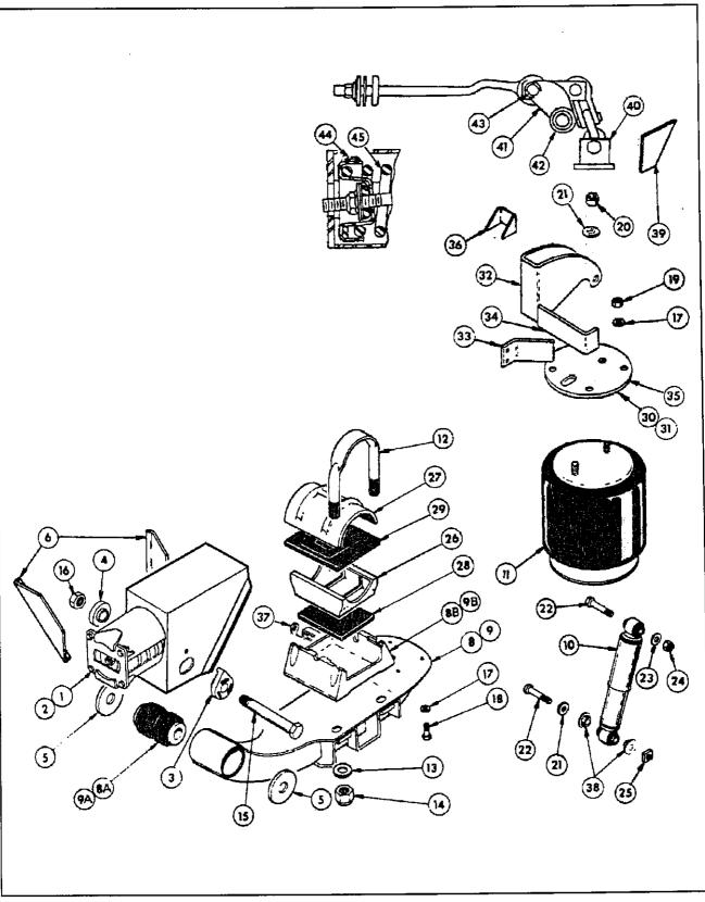
Figure 6-9 Air Ride Suspension (AR-95, AR-955)
