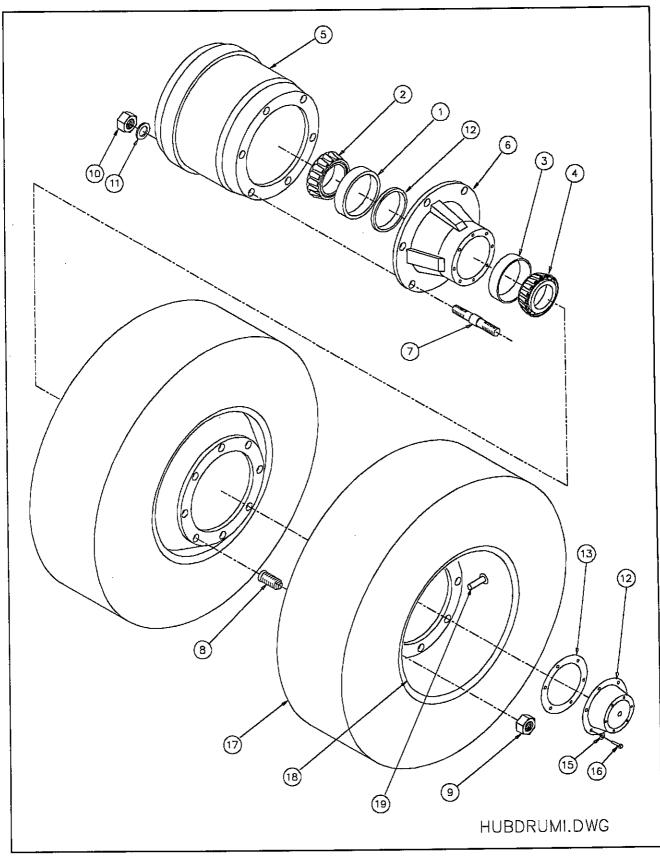
Figure 6-14 Inboard Hub and Drum Assembly
