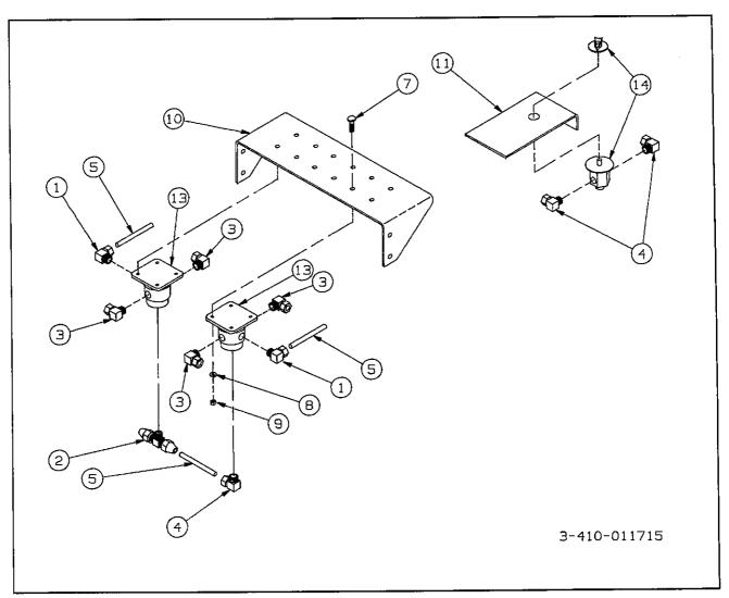
Figure 6-10 Axle Lift Control Assembly
