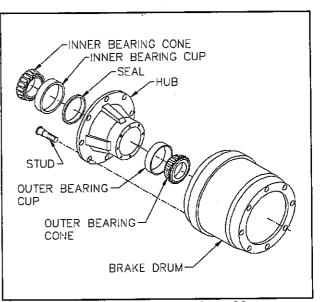
Fig. 4-5 Hub and Drum Assembly
