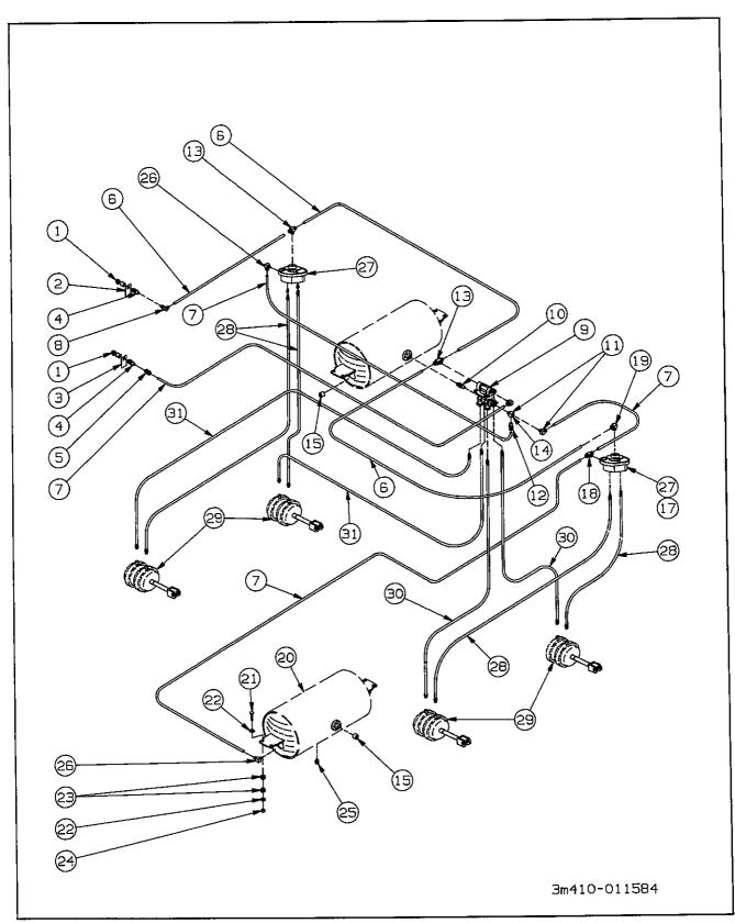
Figure 6-3 Air Brake System, Tandem Axle
