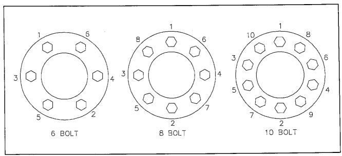
**Figure 4-13 Stud Tightening Sequence**
