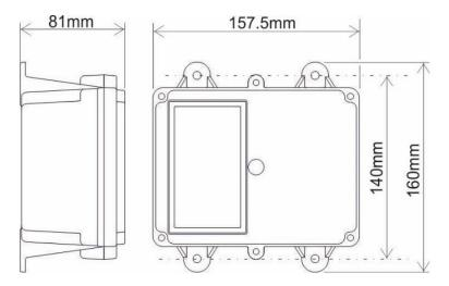
Weight Lid Base Breather Mounting Fixings IP Rating 0.5 lbs (335gms) Clear PC/FR V0 and UV stabilised Black PC V0 and UV stabilised Gortex fitted in base 4 external lugs 5mm (3/16") not supplied IP55
