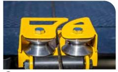
Guide wire or synthetic rope through slot on housing.
