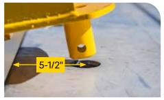
For an aluminum bed, drill a 2" hole 5-1/2" on center from the back edge of the deck and equal distance from the side rails.
