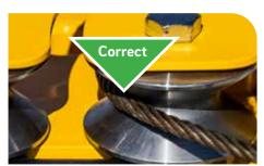
Make sure winch line is centered on sheave prior to winching.
