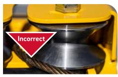
**WARNING!** Failure to align the winch line can cause the rope to slip between the pulley and housing, resulting in damage to both if not corrected.
