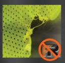
Indistinguishable from the standard polyester mesh, this material is chemically treated to self extinguish after the flame has been removed. The material will melt and drip and does not meet the ANSI requirements for "FR".
