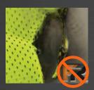
Standard polyester ANSI compliant mesh material ignites when exposed to flame and will continue to burn, melt and drip. It is not recommended for any environment where Arc, sparks or other fire hazards are present.
